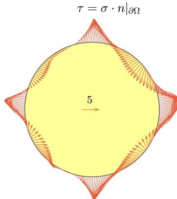
Figure 8: Boundary traction on the disk computed from the stress on  $\partial\Omega$  (scale indicated by the central arrow).
