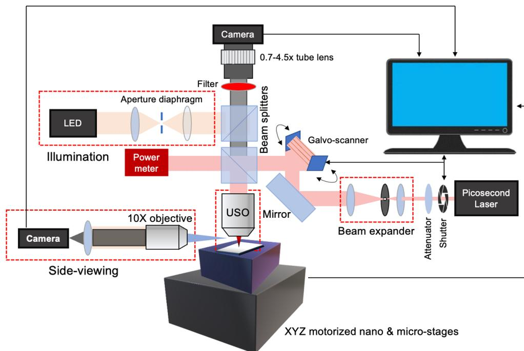
**Figure 1.** Schematic of the SuperNANO system setup.
