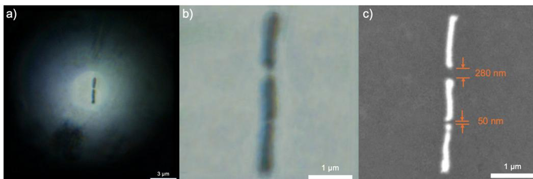
**Figure 8.** Silver nanowire cutting samples under, a) SuperNANO imaging system, b) microscope, c) SEM.
