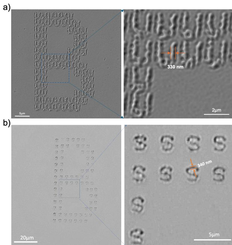
**Figure 6.** Microscope image of a) pixelated 'B' with each pixel is marked with a nano letter 'U', b) pixelated letter 'B' with each pixel is marked with a nano letter 'S'.
