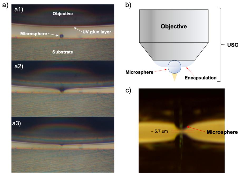
**Figure 2.** a) Production process of USO objective made by microsphere and Plano-Convex lens: a1) objective with UV glue approaching substrate, a2) touching the substrate, a3) detaching from the substrate, b) Unibody Superlens Objective, c) Focusing distance measurement by the side-view microscope system. The substrate acts like a mirror in the image.
