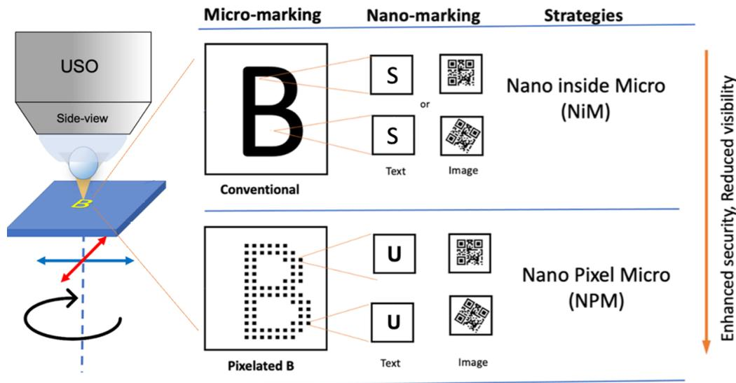
**Figure 3.** Strategies of multi-level laser security marking. NiM (Nano inside Micro): On top of conventional laser marking, adding designed nano-pattern inside. NPM (Nano Pixel Micro): Pixelize micro-marking, replace each pixel with designed nano-pattern.
