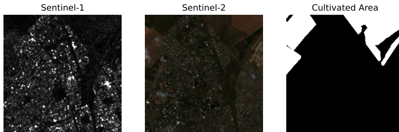
Fig. 4: South Africa Crop Type dataset example. Sentinel-1 shows the grayscale of the VV polarization, while Sentinel-2 shows the RGB of the same area. The mask shows the cultivated area in white.
