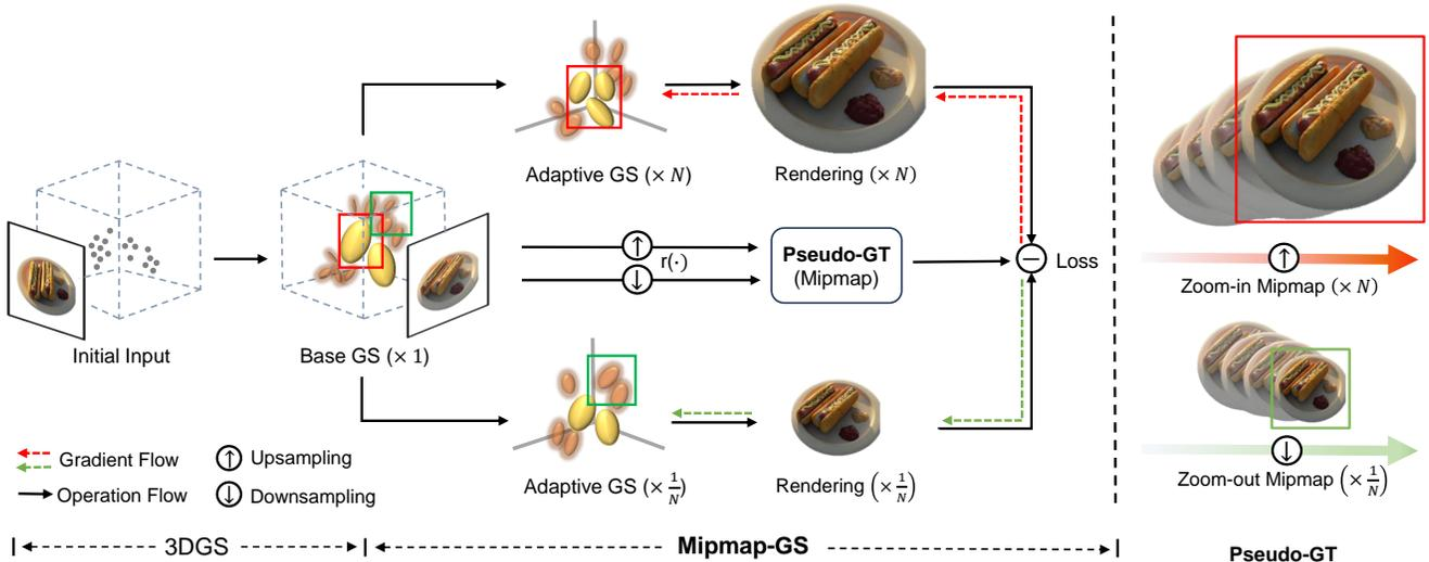
Figure 4. **Pipeline.** We adjust single-scale trained base Gaussians for arbitrary zoom factors supervised by mipmap-like pseudo-GT. The core component is the mipmap proposal module, which constructs scale-specific mipmap by upsampling or downsampling novel views.
