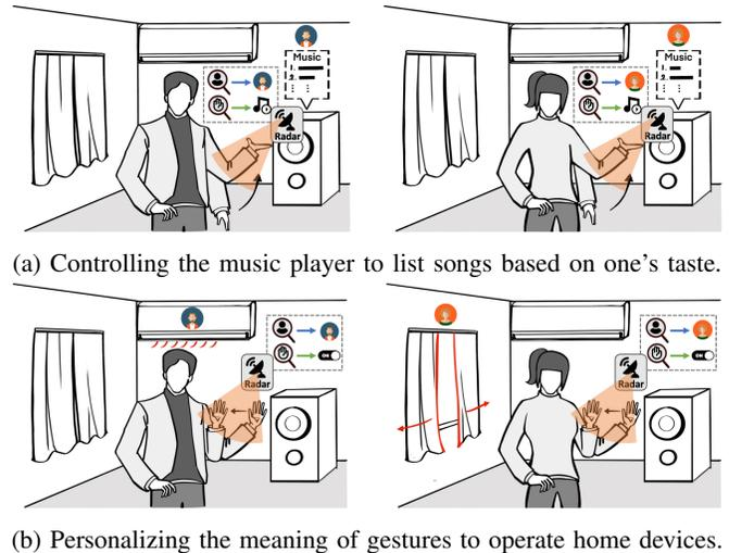
Fig. 1: Potential applications of mmWave-based gesture recognition systems with user identification capability. The identification capability can significantly improve the user experience in interacting with smart devices.
