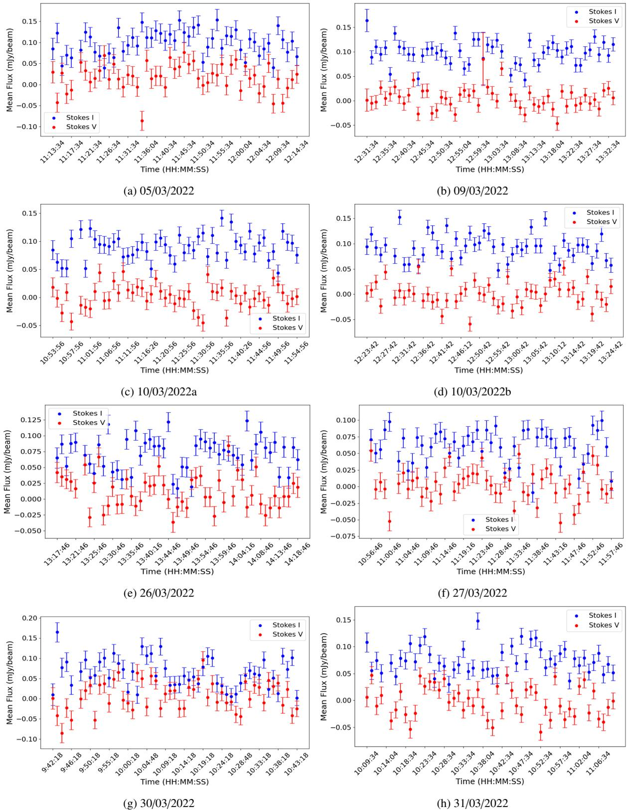
Fig. A.1: 60s time series for all the epochs in Stokes I and Stokes V. These plots have been generated by plotting the real part of amplitude versus time for the target field, using casa task visstat. The error bars represent the statistically calculated standard deviation in the data.
