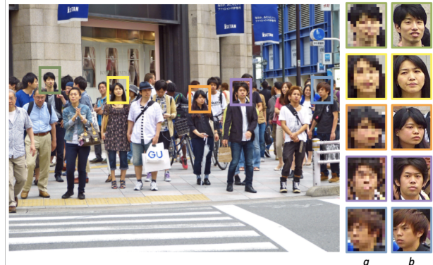
Figure 1: Example objects of interest with (a) ROI of a 320×240 image compressed in processor, (b) ROI of a 2560×1920 image compressed in sensor to 320×240 using HiRISE system.
