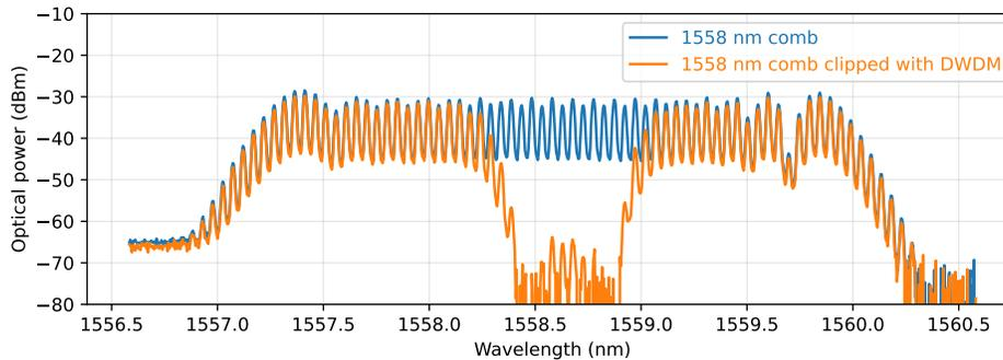
Fig. 7. The spectrum of the 1558 nm comb before (blue) and after (orange) the center of the spectrum is removed using two DWDMs. The use of two DWDMs assures strong suppression of the center comb modes.
