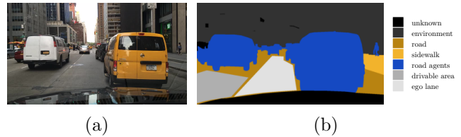
Figure 5: (a) Driving scene from the BDD100K dataset [18]. (b) Respective reduced mask.
