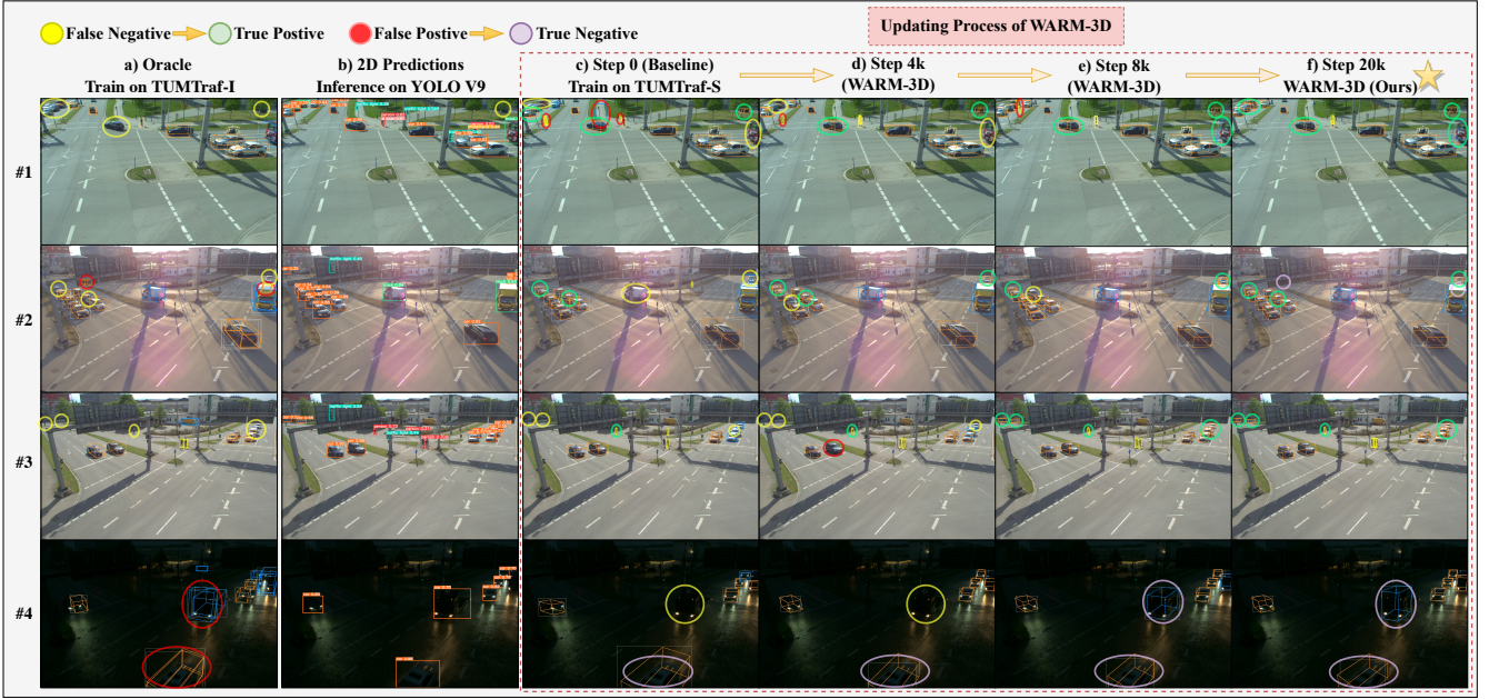
Fig. 5: Visualizations of WARM-3D performance on TUMTraF-I Dataset test set. The WARM-3D in f) method performs even qualitatively better than the oracle method in a). The WARM-3D adaptation process is shown from 0 training steps in c) to 20k training steps in f). It’s evident that the False Negative objects turn to True Positive , while False Positive objects become True Negative in the process.
