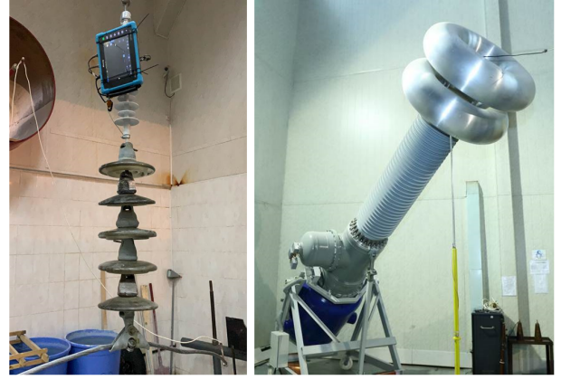
Fig. 4. left - high voltage installation UIV-500 (with voltage level up to 500 kV, load up to 60 kVA, and sustained short circuit current 0.3 A); right - insulator string under testing.
