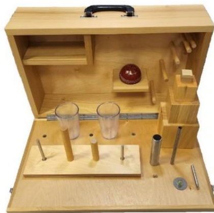
Figure 4: The Action Research Arm Test kit: Using the ARAT kit to evaluate the functionality of the developed 6DOF prosthesis and reliability of the machine learning model
