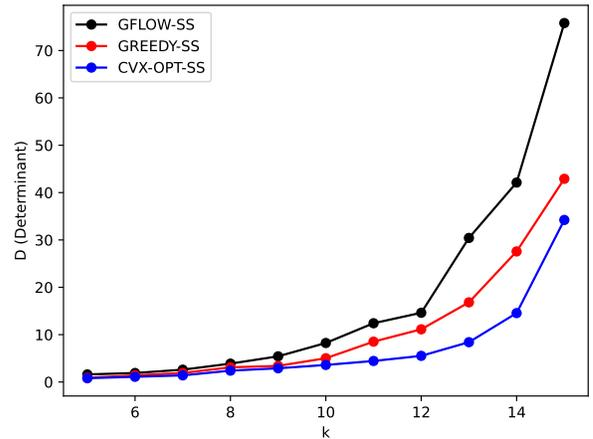
Fig. 2. Comparison of the performance of **GFLOW-SS**, **GREEDY-SS** and **CVX-OPT-SS** for the problem of selecting  $k$  sensors out of 100. The parameter  $k$  ranges from 5 to 15. Each point corresponds to the average performance of the respective approach over 8 different instantiations. The **GFLOW-SS** approach is trained for 40000 root-to-leaf MDP trajectories for every instantiation of the problem. This corresponds to  $40000 \times k$  gradient descent steps.
