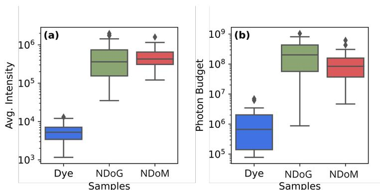
**FIG. S8.** Measured fluorescence enhancement: Average intensity enhancement **a** and total photon budget enhancement **b**. From each measured time-series, the 'ON' spectra are extracted by subtracting the background collected after the fluorophore has bleached. Summation of counts from the average 'ON' spectra gives **a**, while summation of all pixel intensities for the entire 'ON' duration gives **b**.
