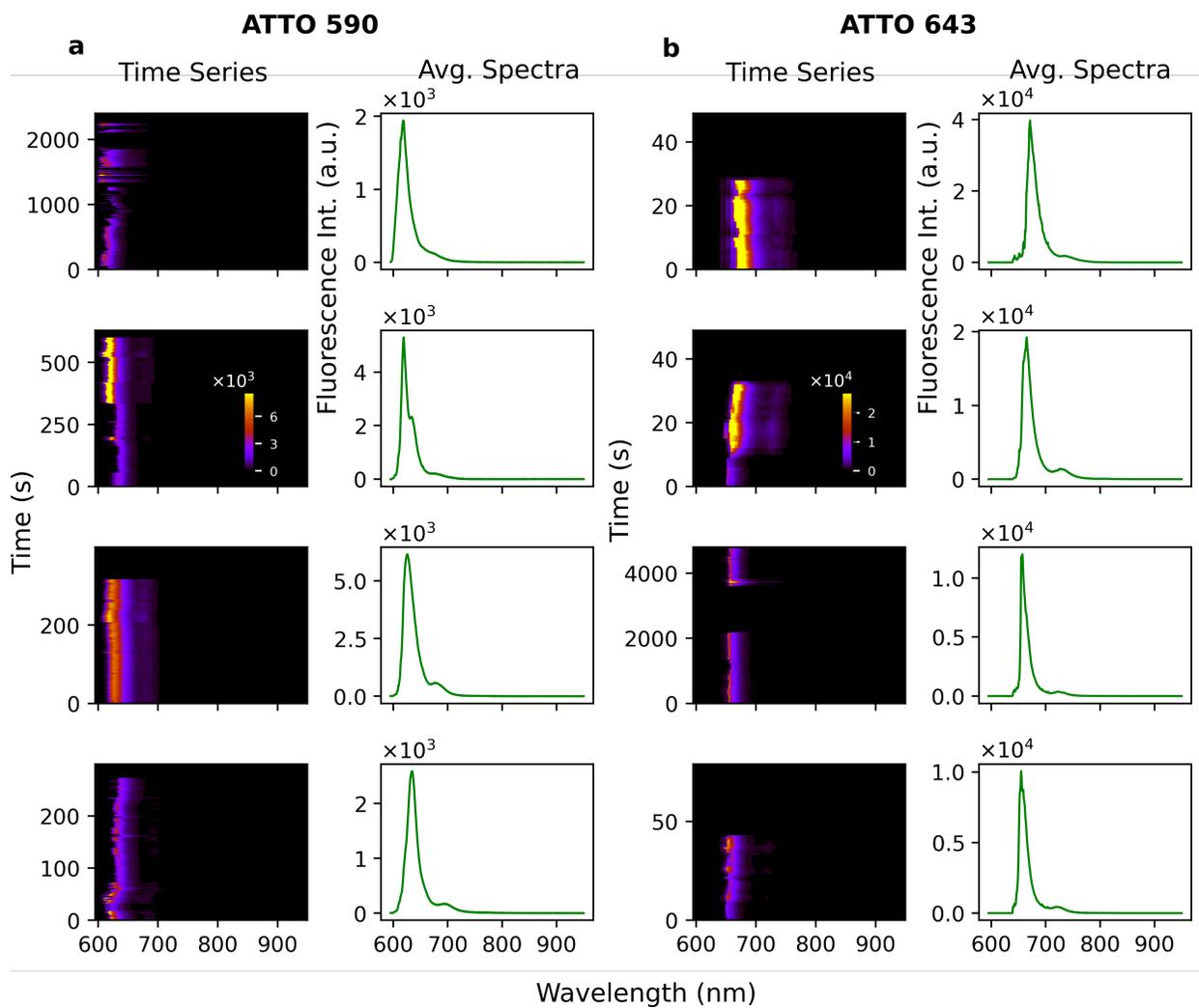
**FIG. S12.** Nano-dimer on glass spectra: Example time-series and average 'ON' spectra of single NDoG containing fluorophores at 4 K. ATTO 590 examples are shown in **a** and ATTO 643 in **b**.
