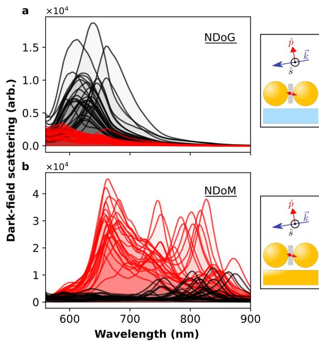
**FIG. S2.** Room-temperature dark-field scattering: Dark-field scattering spectra of individual NDoG **a** and NDoM **b** cavities. Each nanoparticle is excited by  $s$ - and  $p$ -polarized white light. An excitation angle of  $81^\circ$  and collection NA of 0.9 are used.
