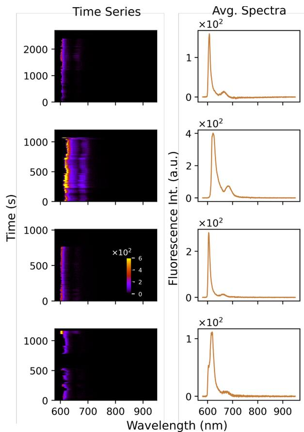
**FIG. S11.** Nano-particle on glass spectra: Example time-series and average 'ON' spectra from a few NPOG containing ATTO 590; measurements at 4 K.
