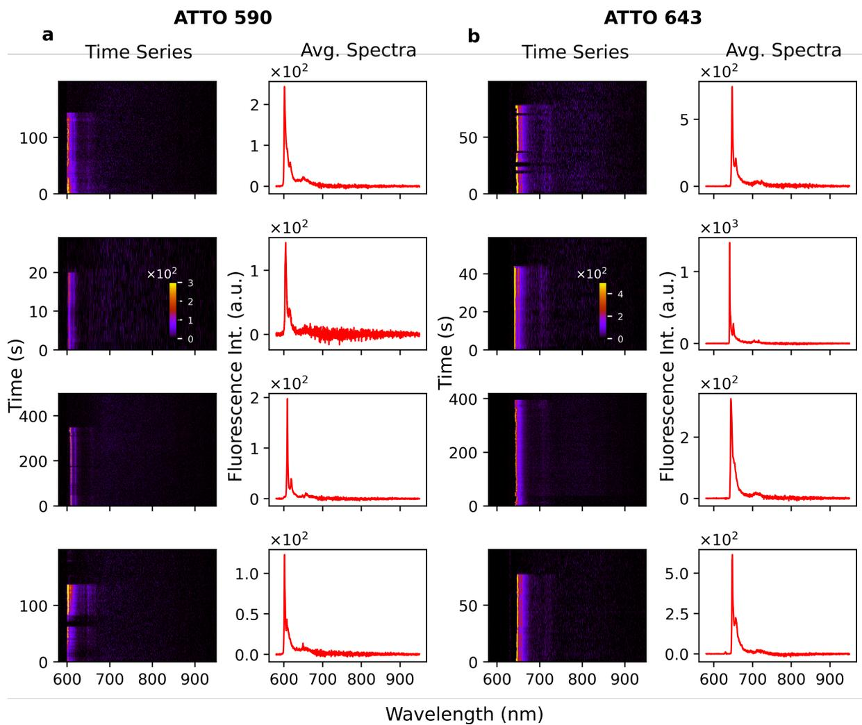
**FIG. S10.** Fluorophore spectra: Example time-series and average 'ON' spectra for single fluorophores, ATTO 590 in **a** and ATTO 643 in **b**, measured at 4 K.
