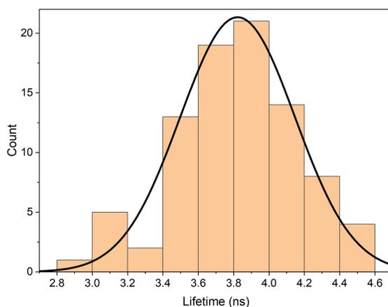
**FIG. S19.** Fluorophore lifetime measurement. DNA origami with ATTO590 on glass in air is measured at ambient conditions. The lifetime histogram of all measured points is plotted, and fit to a Gaussian, giving a mean lifetime of 3.8 ns. Since the quantum yield is characterised by the manufacturer to be 80%, the radiative lifetime is estimated as 4.7 ns
