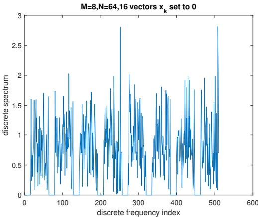
Fig. 2. Spectrum of a VOFDM signal of length 512 with  $M = 8$  and  $N = 64$ , and the first 16 information symbol vectors  $\mathbf{x}_k$ ,  $0 \leq k \leq 15$ , are set to 0.
