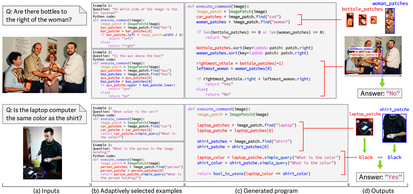
Figure 7: Qualitative examples. (a) Input of questions and images. (b) Adaptively selected example code snippets. Each compressed prompt involves three or four snippets, and two of them are shown. These examples are fed into LLM with the compressed API definition in Figure 6. (c) Generated Python program for question answering. (d) Visualization of intermediate outputs to derive the answer.
