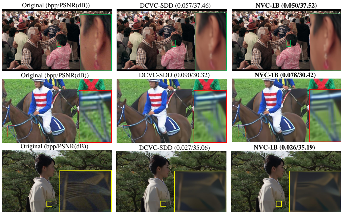
Fig. 9. Subjective quality comparison between our proposed large model—NVC-1B and its small baseline model—DCVC-SDD [32] on the 5th frame of the MCL-JCV videoSRC14 sequence, the 7th frame of the HEVC Class D RaceHorses sequence and the 17th frame of the HEVC Class B Kimono1 sequence.
