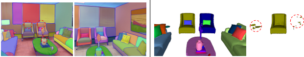
Figure 2. Failure cases of SOTA. Using SAM independently on each image precludes corresponding objects between views (Left). Even if one were to solve this correspondence problem, slight errors in SAM output mean that the same object may be segmented differently in the different views (e.g., the top of the vase is included in the vase segment in the left image but not the right). Even with good segmentations, prior work such as ObjectSDF++ [31] introduces floating artifacts, especially those hidden behind other objects (Right).
