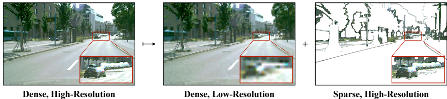
Fig. 1: Processing dense high-resolution inputs is computationally expensive. In this paper, we propose an alternative approach by integrating dense low-resolution and sparse high-resolution inputs, which provide complementary information about the overall scene layout and intricate object details. Leveraging the lower resolution and sparsity of these inputs allows for more efficient processing.
