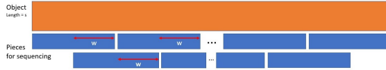
Figure 1: Object recovery from pieces: Due to objects obscuring each other, we cannot hope to see all s pixels of the orange object at once, but so long as we see the blue pieces shown in this figure, i.e., ones with at least w pixels overlap, we can reconstruct the object.
