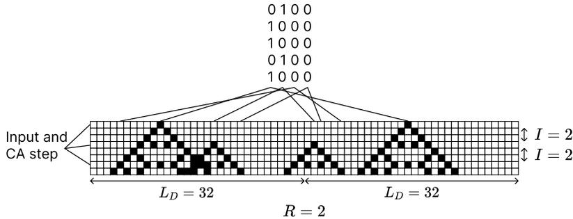
FIGURE 10: ReCA example showing  $R$ ,  $I$  and  $L_d$ . Additionally, the top streams is an example of how input is encoded temporarily into the reservoir.
