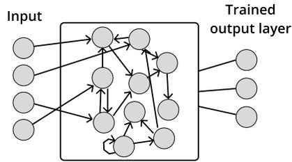
FIGURE 9: Basic network Architecture of an ESN.
