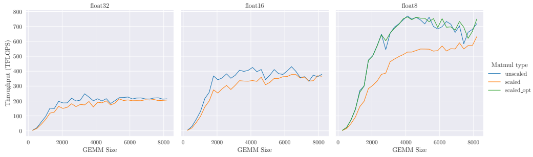
Figure 18: Square matrix multiplication throughput in TFLOPs with and without scaling factors applied to the output across 32-, 16-, and 8-bit float dtypes on NVIDIA H100 PCIe. Naive implementation in PyTorch.
