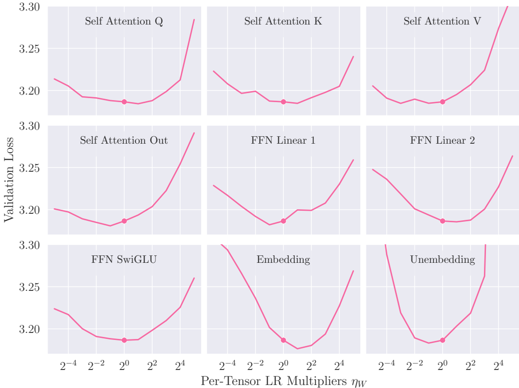
Figure 8: Independently varying per-tensor learning rate multipliers \eta_W , using the u- \mu P model of width 256 from Figure 1 with optimized global learning rate 2^{1.5} as the starting point. Where applicable, the same multiplier is used for tensors of the same name across transformer layers. Each subplot fixes all but one multiplier at 1, therefore the midpoint of each subplot is precisely the u- \mu P 256 model from Figure 1.
