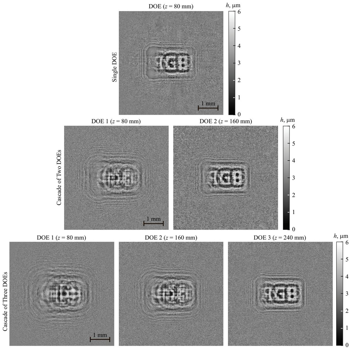
Figure 3: Calculated microrelief height functions of the designed single DOE (top row), cascade of two DOEs (middle row), and cascade of three DOEs (bottom row).
