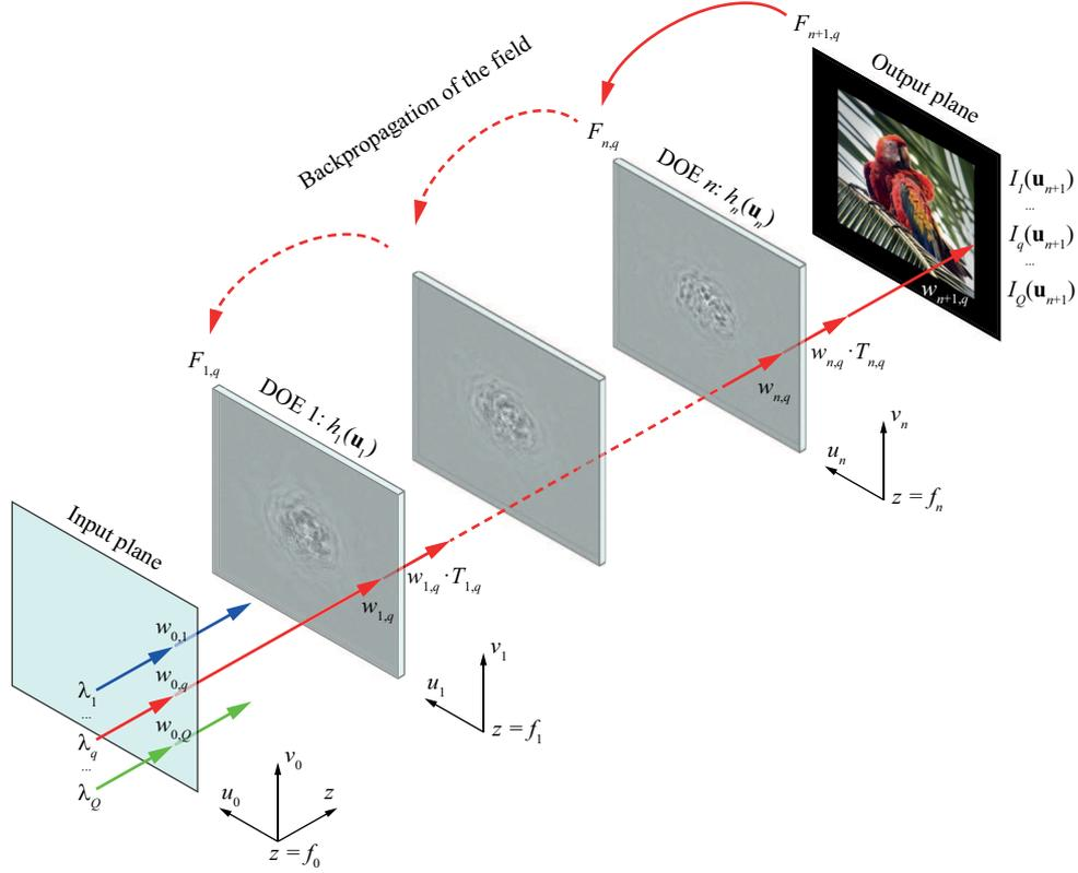
Figure 1: Geometry of the problem of calculating a cascaded spectral DOE.
