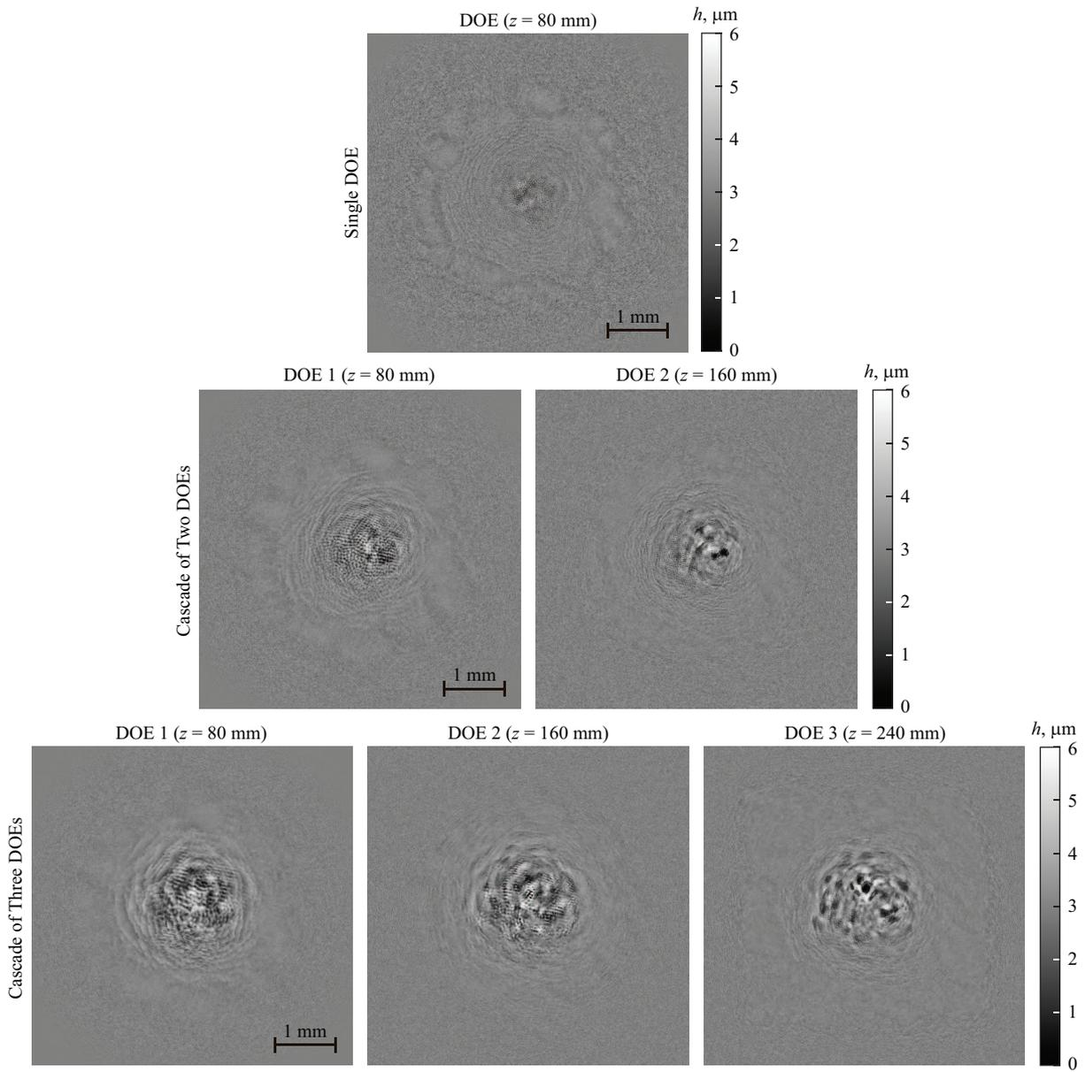
Figure 6: Calculated microrelief height functions of the designed single DOE (top row), cascade of two DOEs (middle row), and cascade of three DOEs (bottom row) generating a color image of parrots.
