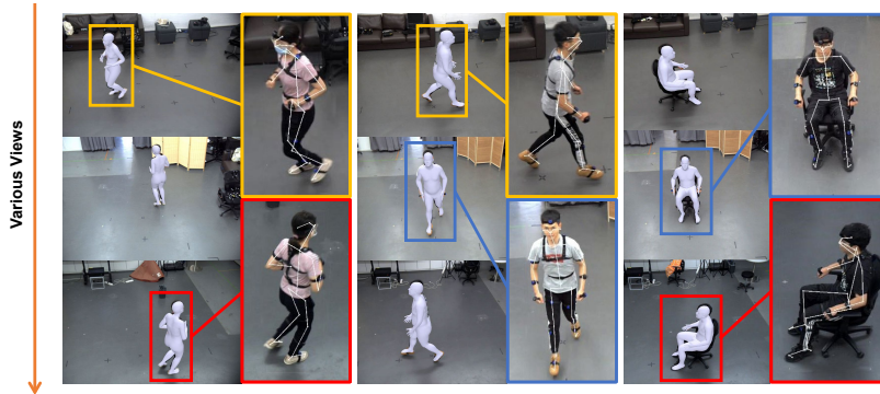
Fig. 6: Qualitative results from single-subject motion capture data collection. Results of 3D mesh and the corresponding re-projected full-body 2D joints from various views.
