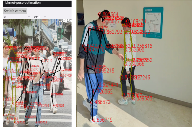
Fig. 6: Visualization of the Android UI on smartphones with the DIR-BHRNet for real-time MPPE. For more details, please refer to the video description 1 .
