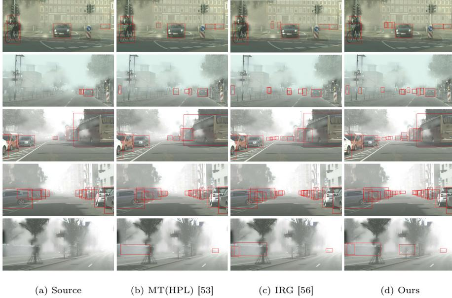
**Fig. 6:** Additional qualitative results for Cityscapes [10]  $\rightarrow$  Foggy Cityscapes [48]. Bounding boxes in **red** refer to the prediction. *Zoom in for best view.*
