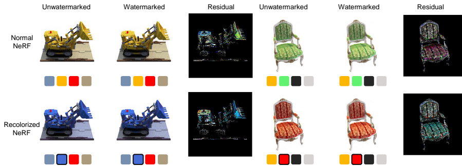
Fig. 5: Residual maps for NeRF renderings before and after palette-based recolorizations. The first row shows the residual maps before palette-based recolorizations. The second row shows the residual maps after palette-based recolorizations. Each residual map shows the differences between the unwatermarked renderings and watermarked renderings by GeometrySticker.
