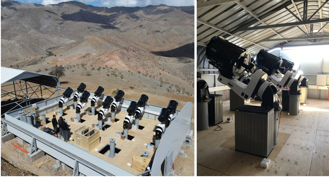
Figure 1. (Left) 7DT overview. Currently, 7DT is under construction with 10 of 20 units operational. (Right) Specific view of telescope unit. Each telescope unit is connected to the TCC located below the telescope unit. For more detail of 7DT, see ( https://gwuniverse.snu.ac.kr/research/7dt )
