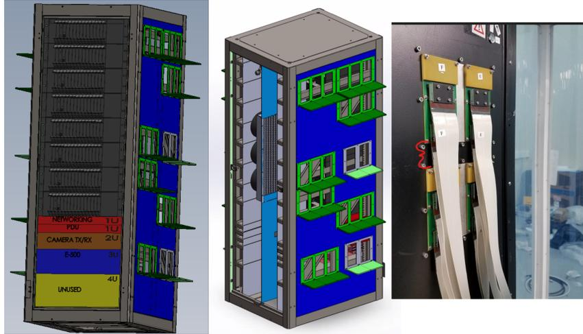
Figure 9. Management of MEMS ribbon cables. Feed through connectors will be placed on the outside rack #1 housing the MEMS electronics. The right photo shows such a system in operation on the current MagAO-X instrument.
