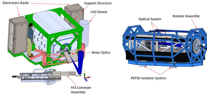
Figure 1. Overview of the Mechanical Design of GMagAO-X
