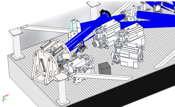
Figure 6. The parallel DM is shown rendered in the opto-mechanical design of GMagAO-X.
