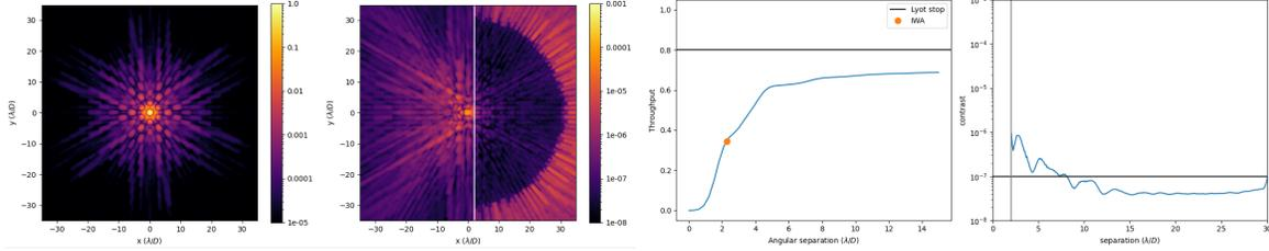
Figure 7. Preliminary PAPLKEC coronagraph design for GMagAO-X. This design is for a 20% bandwidth. Left shows the PSF. Middle-left shows the dark hole (with no residual atmosphere). Middle-right shows the throughput curve, with inner working angle of  $2.3 \lambda/D$  defined at 50% throughput. Right shows raw contrast vs. separation.
