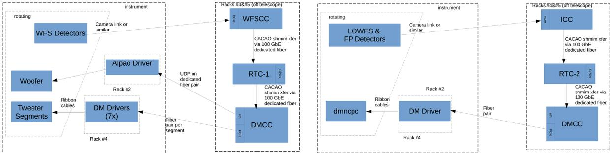
Figure 10. The distributed real-time control system of GMagAO-X
