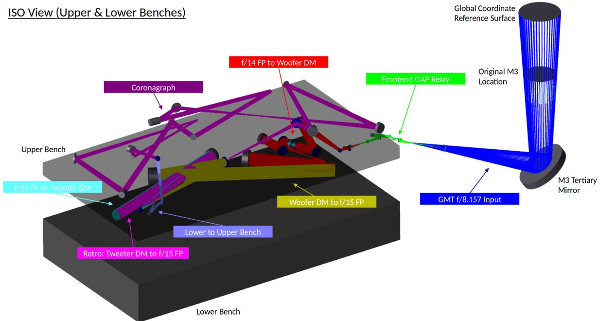
Figure 4. The Optical Design of GMagAO-X
