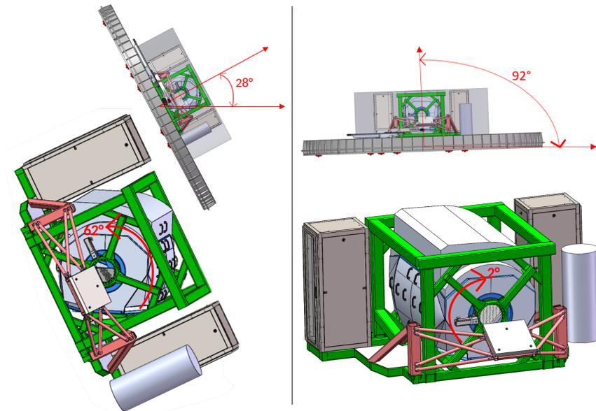
Figure 2. Gravity Invariance: The optical table of GMagAO-X is rotated to be gravity invariant during operation.
