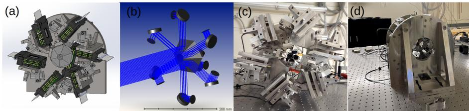
Figure 5. The Parallel DM Concept: the large-segment primary mirror of GMT motivates using a segmented DM with 3000 actuators per segment. (a) Mechanical Design. (b) Optical Design. Note the crossed folds for polarization control. (c) & (d) Prototype assembled and tested on the HCAT testbed at the University of Arizona.
