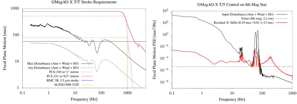
Figure 11. Left: GMagAO-X tip/tilt stroke requirements. Right: GMagAO-X tip/tilt suppression on an 8th mag star
