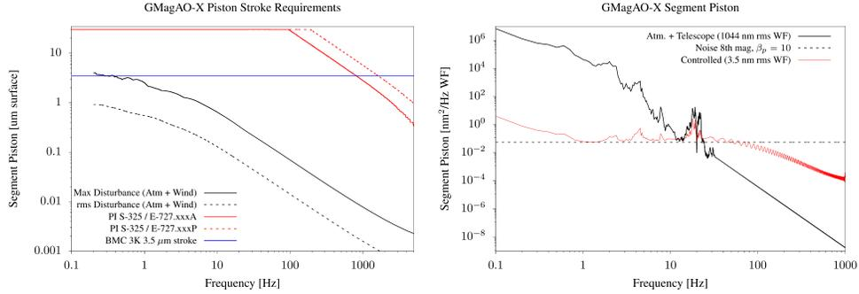
Figure 12. Left: GMagAO-X segment piston stroke requirements. Right: GMagAO-X segment piston suppression on an 8th mag star
