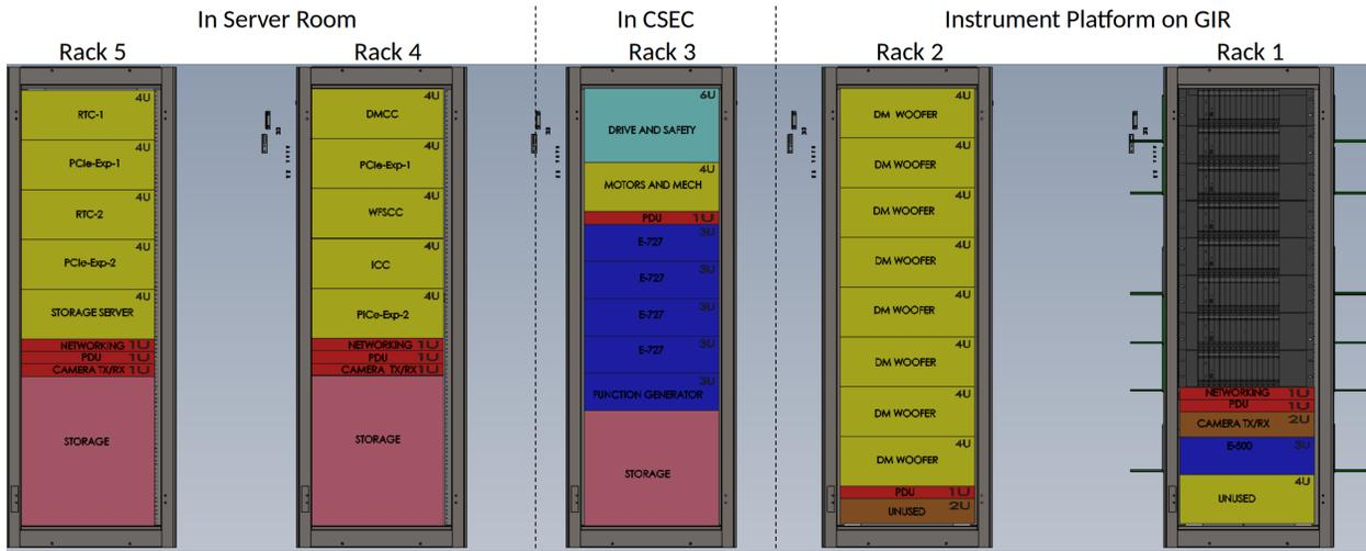
Figure 8. The equipment racks used to house GMagAO-X electronics. Rack 1 houses the 8 MEMS driver (7x for the parallel DM tweeter, 1x for the NCPD DM and image acquisition hardware). Rack 2 houses the 32 U ALPAO DM 3228 driver. Rack 3 houses motion control and drivers for the parallel DM PTT stages. Racks 4 and 5 are off the telescope and house the distributed real-time control computer system.
