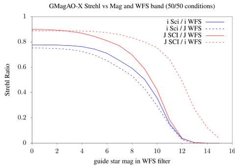
Figure 13. Strehl ratio vs. guide star magnitude for GMagAO-X, for different combinations of WFS and science wavelengths.
