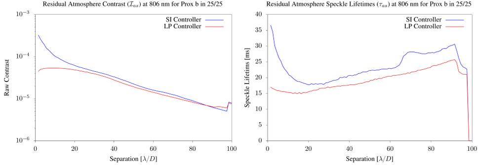
Figure 14. Left: GMagAO-X residual atmospheric instantaneous contrast. Right: GMagAO-X residual atmosphere speckle lifetime. Blue is for the simple integrator controller, and red is for the ideal linear predictor controller.
