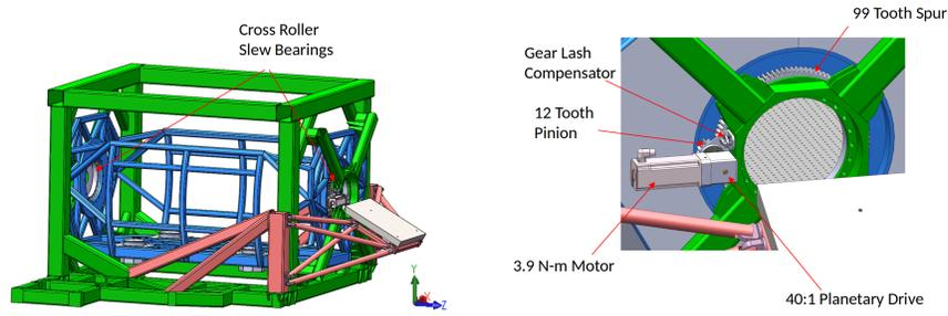
Figure 3. The Rotation Mechanism of GMagAO-X
