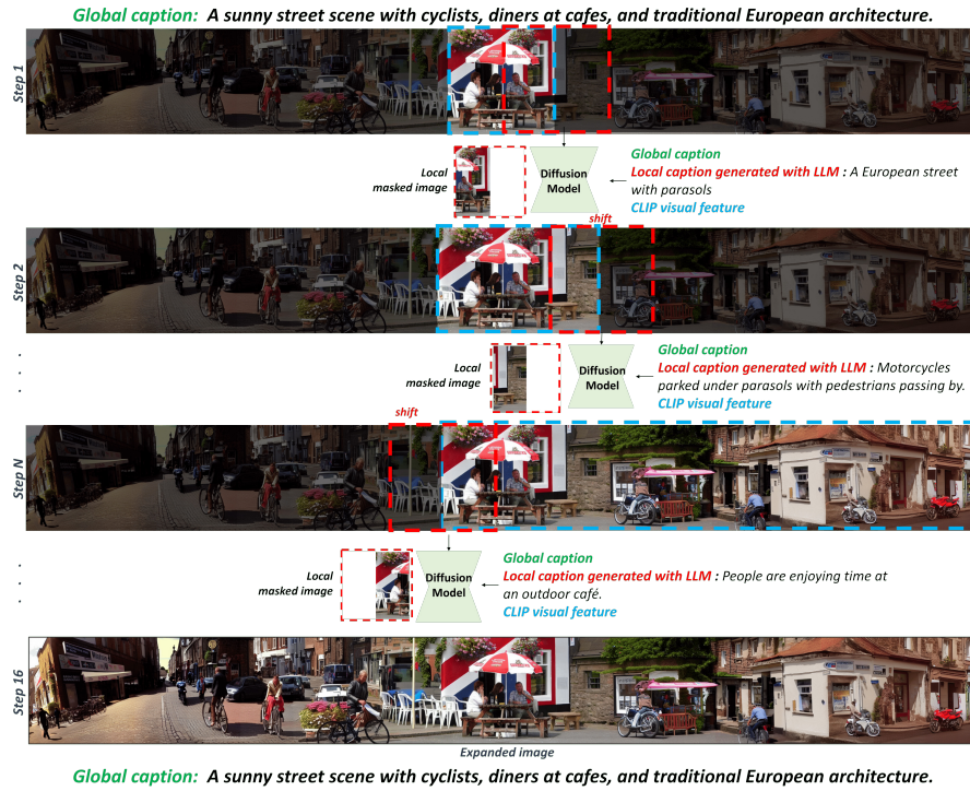
Fig. 5: Inference Pipeline. We expand the local image autoregressively by conditioning on the global caption, local caption generated by the LLM and the visual feature. The figure image is generated with a 16-step process ( 4608 \times 512 ). The red box is a local masked image, and the blue box is an expanded global image that is input into the CLIP image encoder.
