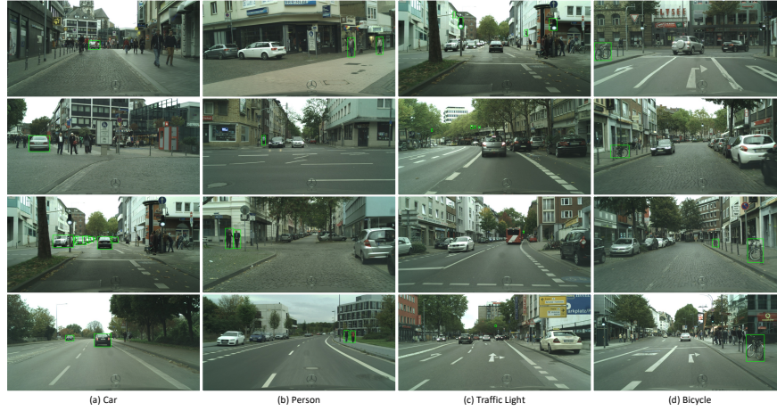
Fig. 5: Detection results on Cityscapes unlabeled images Faster R-CNN model trained on 1/16 labeled data in Cityscapes dataset and confidence \geq 0.9 . From left to right: Car, Person, Traffic Light, Bicycle.
