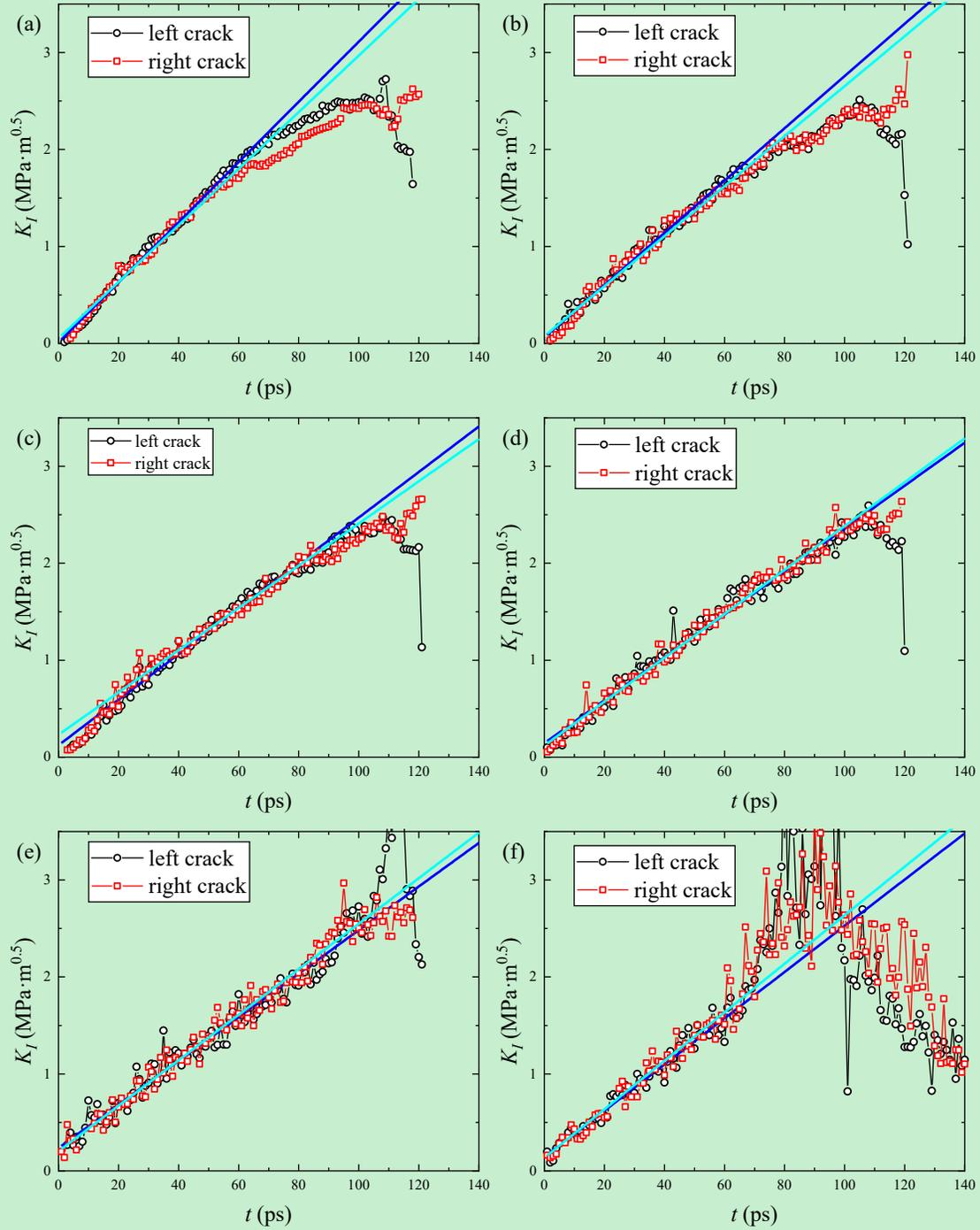
**Fig. 11.** The DSIF  $K_I(t)$  as a function of time  $t$  for the  $\Sigma 3(109.5)$  specimen at (a)  $T = 0.01T_m$ ; (b)  $T = 0.1T_m$ ; (c)  $T = 300\text{ K}$ ; (d)  $T = 0.3T_m$ ; (e)  $T = 0.5T_m$ ; (f)  $T = 0.7T_m$ . For each panel, the blue and cyan curve are the linearly fitted to the left (black) and right (red) crack data points, respectively.
