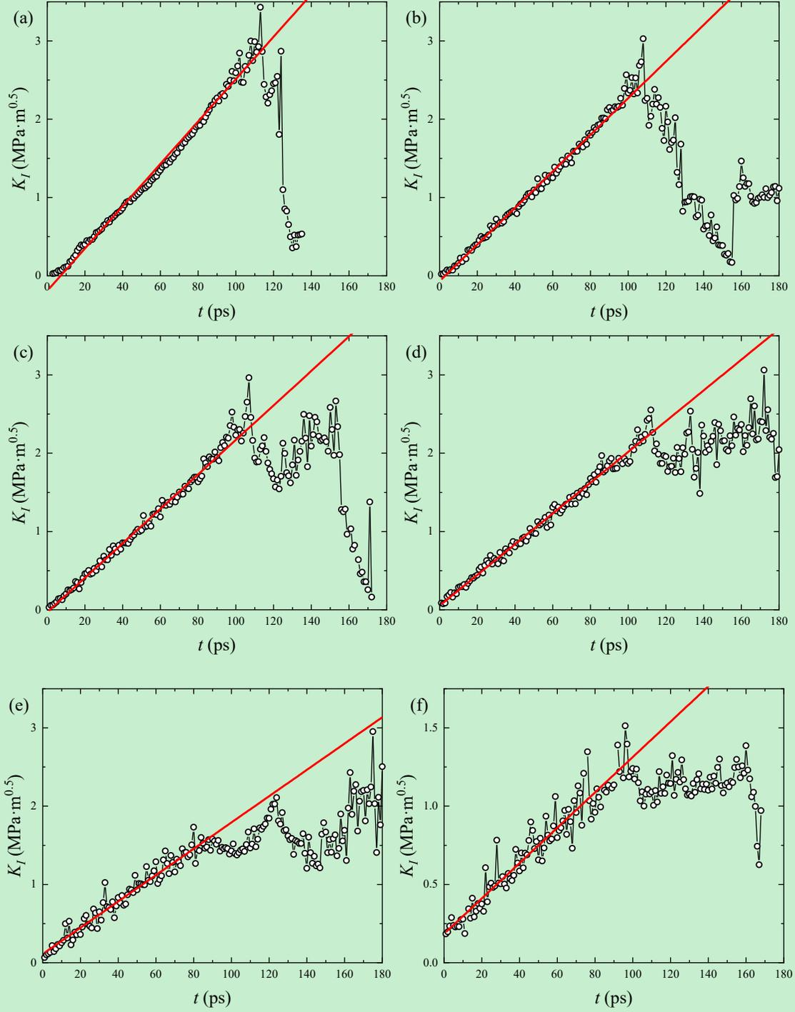
**Fig. 10.** The DSIF  $K_I(t)$  as a function of time  $t$  for the left crack of the  $\Sigma 11(50.50)$  specimen at (a)  $T = 0.01T_m$ ; (b)  $T = 0.1T_m$ ; (c)  $T = 300\text{ K}$ ; (d)  $T = 0.3T_m$ ; (e)  $T = 0.5T_m$ ; (f)  $T = 0.7T_m$ .
