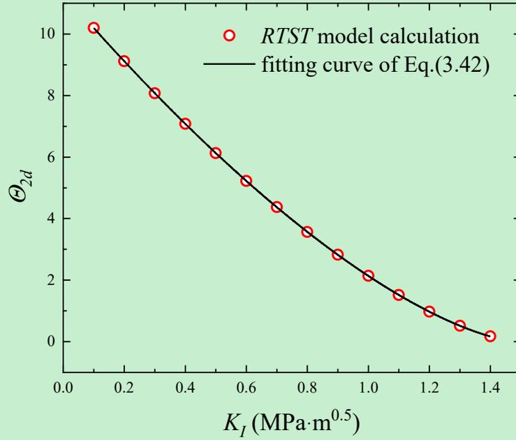
**Fig. 17.** The schematics of the  $\theta_{2d}(K_I)$  v.s.  $K_I$  fitting procedure. The red circle represents the theoretical predictions via the **RTST** and **PRB** models, while the black curve is obtained by fitting the theoretical results to **Eq.(3.42)**.
