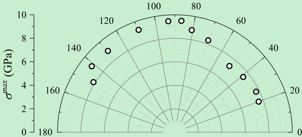
**Fig. 4.** The maximum tensile stress  $\sigma^{max}$  as a function of the GB tilt angle  $\theta$  for tests at 300 K.
