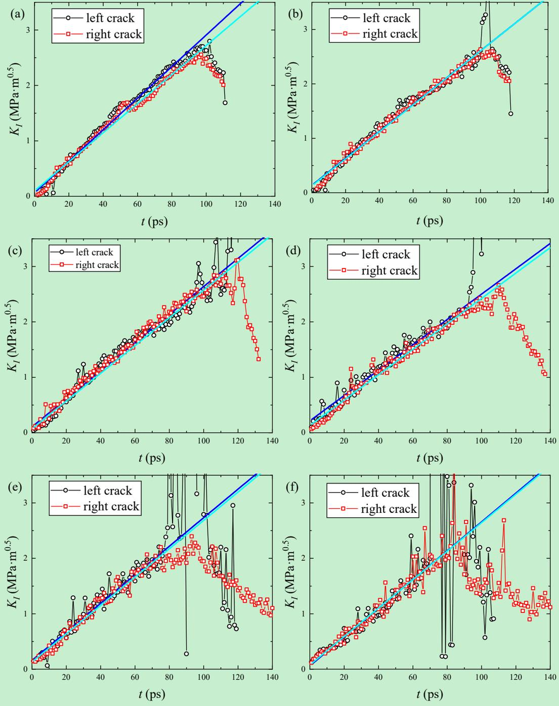
**Fig. 12.** The DSIF  $K_I(t)$  as a function of time  $t$  for the  $\Sigma 9(141.6)$  specimen at (a)  $T = 0.01T_m$ ; (b)  $T = 0.1T_m$ ; (c)  $T = 300$  K; (d)  $T = 0.3T_m$ ; (e)  $T = 0.5T_m$ ; (f)  $T = 0.7T_m$ . For each panel, the blue and cyan curve are the linearly fitted to the left (black) and right (red) crack data points, respectively.
