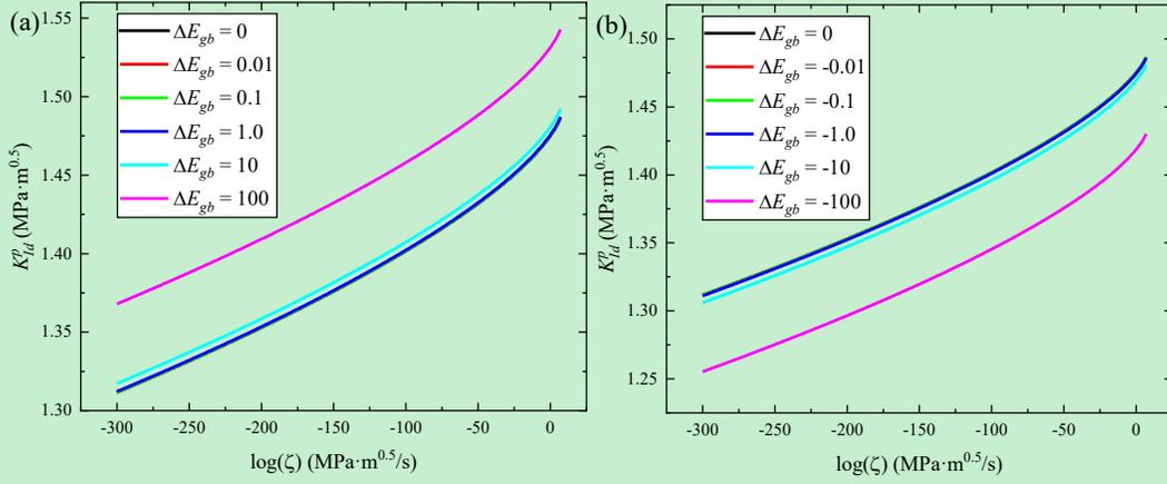
**Fig. 20.** The  $K_{Id}^p$  v.s.  $\zeta$  relation with the scaling factor  $s_0 = 5b$  (with the angle  $\theta = 0.3\pi$ ) for cases with different  $\Delta E_{gb}$  (in the unit of  $\text{GPa}\cdot\text{\AA}^2$ ). (a) for  $\Delta E_{gb} > 0$ ; (b) for  $\Delta E_{gb} < 0$ .
