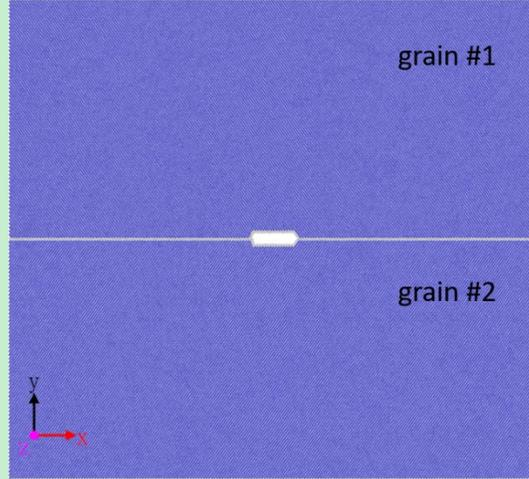
**Fig. 1.** Schematics of the bicrystalline specimen with a through-thickness crack at the GB. The atoms are colored by the a-CNA parameter, with the bcc atoms as blue and disordered as white.
