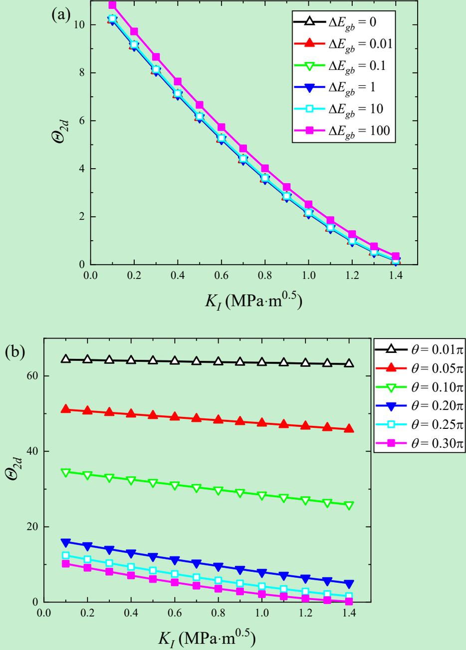
**Fig. 16.** The normalized activation energy for dislocation nucleation from the crack-tip  $\Theta_{2d}$  as a function of the applied Mode-I SIF  $K_I$ . (a) under various GB energy change  $\Delta E_{gb}$  (due to dislocation emission) values, with the angle between the slip plane and the crack plane  $\theta = 0.3\pi$ . The unit of the GB energy change  $\Delta E_{gb}$  is  $\text{GPa}\cdot\text{\AA}^2$ . (b) under various  $\theta$  values, with the GB energy change  $\Delta E_{gb} = 0$ .
