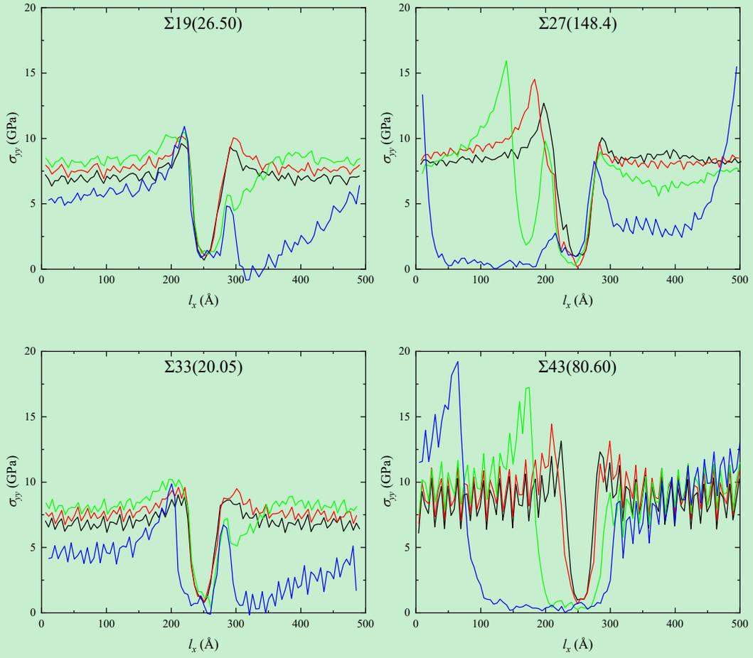
**Fig. 9.** Tensile stress profile at 300 K along the  $x$ -axis direction under different strains  $\epsilon = 4.5\%$ ,  $5.0\%$ ,  $5.5\%$  and  $6.0\%$ , with the valley at the center of the  $x$  dimension indicates the position of the crack.
