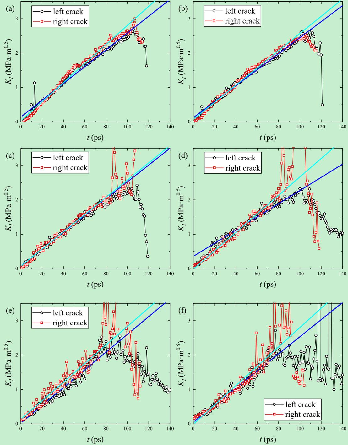
**Fig. 14.** The DSIF  $K_I(t)$  as a function of time  $t$  for the  $\Sigma 27(148.4)$  specimen at (a)  $T = 0.01T_m$ ; (b)  $T = 0.1T_m$ ; (c)  $T = 300 \text{ K}$ ; (d)  $T = 0.3T_m$ ; (e)  $T = 0.5T_m$ ; (f)  $T = 0.7T_m$ . For each panel, the blue and cyan curve are the linearly fitted to the left (black) and right (red) crack data points, respectively.
