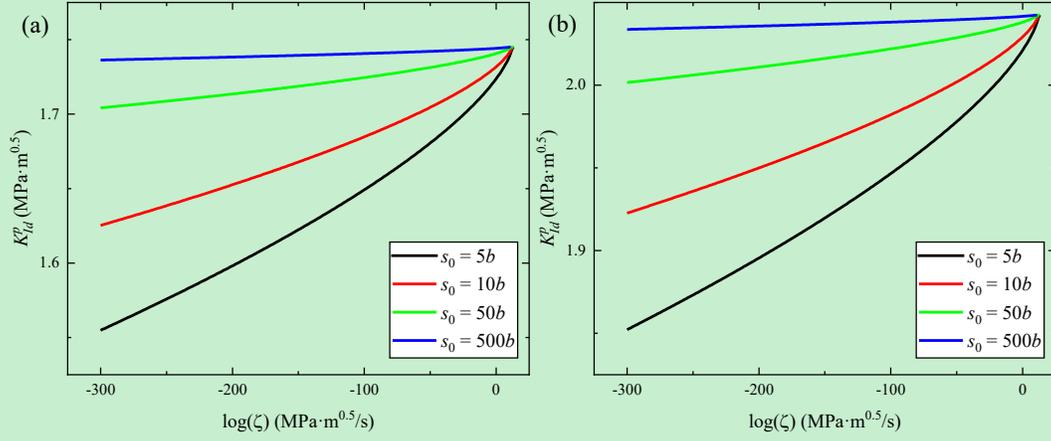
**Fig. 18.** The  $K_{Id}^p$  v.s.  $\zeta$  relation with various scaling factor  $s_0$  with the angle  $\theta = 48.5^\circ$  and, (a)  $\Delta E_{gb} = 100 \text{ GPa} \cdot \text{\AA}^2$ , (b)  $\Delta E_{gb} = 600 \text{ GPa} \cdot \text{\AA}^2$ .
