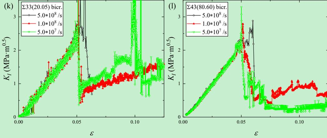
**Fig. 19.** The dynamic Mode-I SIF  $K_I$  of the left crack-tip as a function of the strain  $\varepsilon$  for 12 different bicrystals under different loading rates ( $\dot{\varepsilon} = 5.0 \times 10^8, 1.0 \times 10^8, 5.0 \times 10^7$  /s, respectively) with the environmental temperature  $T = 300$  K.
