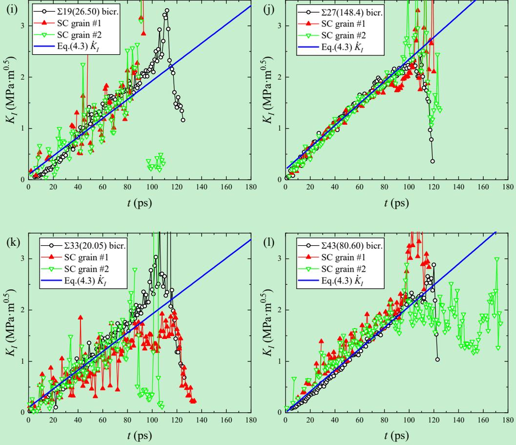
**Fig. 15.** The dynamic Mode-I SIF  $K_I(t)$  of the left crack-tip as a function of the time  $t$  for 12 different bicrystals and 24 corresponding single crystals with the environmental temperature  $T = 300$  K and loading rate  $\dot{\epsilon} = 5.0 \times 10^8$  /s. The blue line is theoretically evaluated by Eq.(4.3) based on the anisotropic elasticity (see details in [Table B1](#) in [Appendix B](#)).
