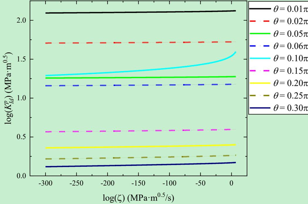
**Fig. 21.** The  $K_{Id}^p$  v.s.  $\zeta$  relation with the scaling factor  $s_0 = 5b$  (with  $\Delta E_{gb} = 0$ ) for cases with different angles  $\theta$ .
