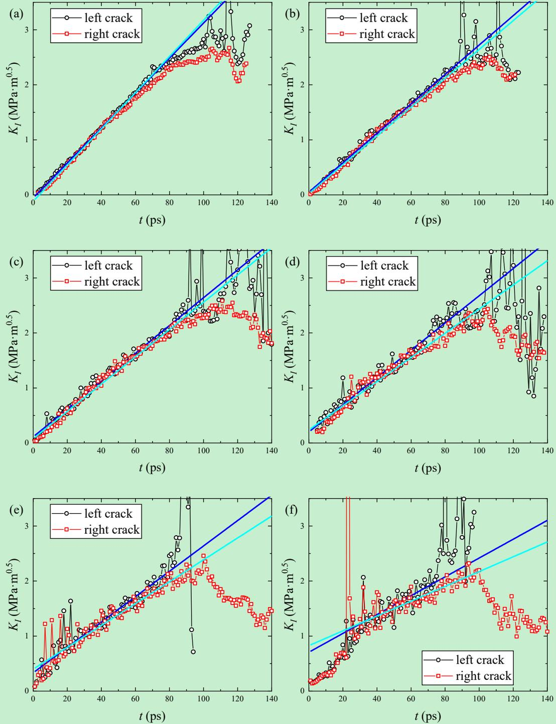
**Fig. 13.** The DSIF  $K_I(t)$  as a function of time  $t$  for the  $\Sigma 11(129.5)$  specimen at (a)  $T = 0.01T_m$ ; (b)  $T = 0.1T_m$ ; (c)  $T = 300 \text{ K}$ ; (d)  $T = 0.3T_m$ ; (e)  $T = 0.5T_m$ ; (f)  $T = 0.7T_m$ . For each panel, the blue and cyan curve are the linearly fitted to the left (black) and right (red) crack data points, respectively.
