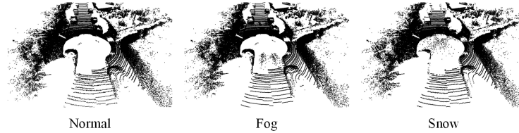
Fig. 1: Visualization of simulated adverse weathers for SemanticKITTI. From left to right: the normal point cloud, the fog point cloud and the snow point cloud are shown one by one.
