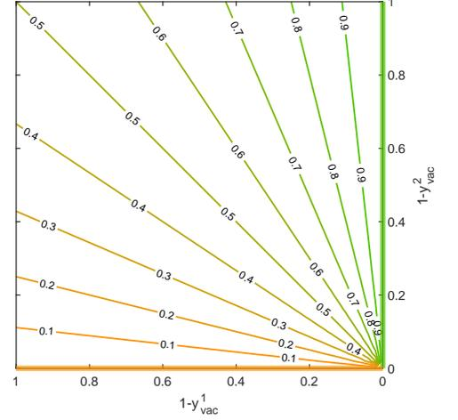
FIG. 5. Mapping of the constitutional square for the (A,Vac)(B,Vac) DEF model, formed by  $(1 - y_{vac}^1) - (1 - y_{vac}^2)$  axes, into the mole fraction composition  $X_B$ .  $X_B = 1$  and  $X_B = 0$  lines are shown by thick green and orange lines, respectively.
