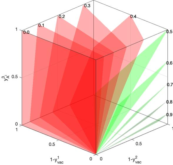
FIG. 8. Mapping of the constitutional cube for the (A,Vac)(B,Vac)(Vac<sup>i</sup>,A<sup>i</sup>) DEF model, formed by  $(1 - y_{\text{vac}}^1) - (1 - y_{\text{vac}}^2) - y_{A^i}^3$ , into the mole fraction composition  $X_B$ . The contour level planes in the constitutional cube are labeled with corresponding  $X_B$  values. Level planes for  $X_B < 0.5$  and  $X_B \geq 0.5$  are colored red and green, respectively.
