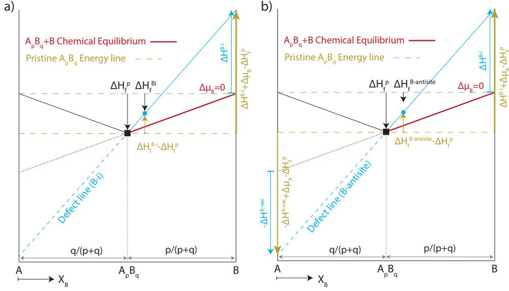
FIG. 3. Formation energy per atom convex hull. Graphical representation of the absolute defect energy for a) B-interstitial and b) B-antisite in an A-A<sub>p</sub>B<sub>q</sub>-B convex hull.
