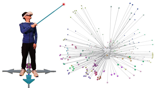
Fig. 4: Left: an illustration of the virtual reality study environment. The user points to a spatial direction when perceiving a vibration on the body. Right: sample data points collected from one participant. Points of the same color are from the same actuator.
