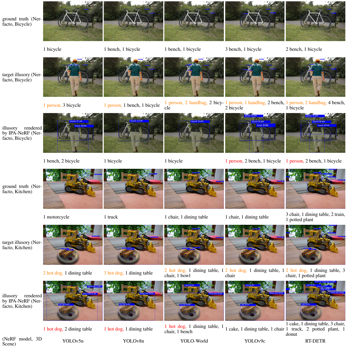
Figure A13. The impact of the IPA-NeRF attack on object detection. Attack epochs: 150, \epsilon : 32, \eta : 0.
