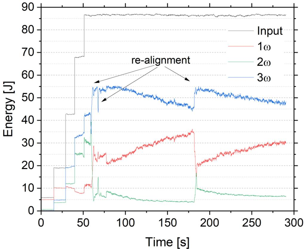
Figure 4 Temporal evolution of the energy of the third harmonic frequency  $3\omega$  together with input energy (1030 nm) and unconverted residual energy on fundamental  $1\omega$  (1030 nm) and second harmonic  $2\omega$  (515 nm) frequencies. Points where crystal phase matching angle was optimized are marked with arrows.
