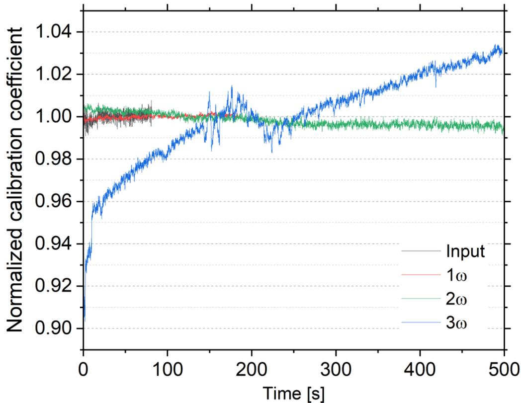
**Figure 2** Temporal evolution of energy meter’s calibration coefficients, while calibration coefficient for input energy ( $1030\text{ nm}$ ) and unconverted fundamental  $1\omega$  ( $1030\text{ nm}$ ) stabilized in order of tens of seconds, the second harmonic  $2\omega$  ( $515\text{ nm}$ ) took hundreds of seconds and the third harmonic  $3\omega$  ( $343\text{ nm}$ ) didn’t stabilize at all.
