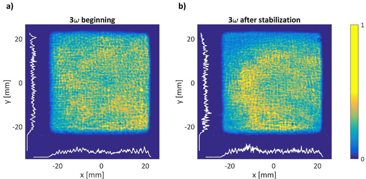
**Figure 7** Beam profile on third harmonic frequency (343 nm) with energy of  $>50$  J at the repetition rate of 10 Hz in the beginning of the experiment (a) and after oven temperature stabilization after 90 minutes (b). The color bar was adjusted to better show the intensity variation in the beam in the presence of hot spots that affected the normalization.
