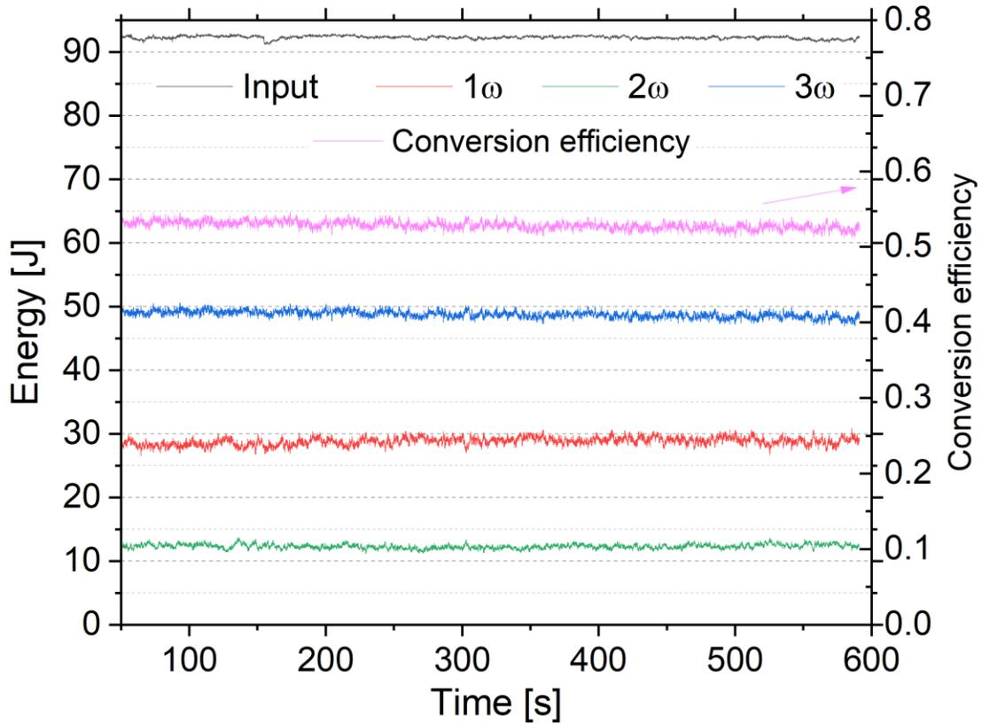
**Figure 6** Temporal evolution of the energy of the third harmonic frequency  $3\omega$  (343 nm) together with input energy (1030 nm) and unconverted residual energy on fundamental  $1\omega$  (1030 nm) and second harmonic  $2\omega$  (515 nm) frequencies after SHG oven temperature stabilization and fine tuning of the SHG LBO phase matching angle. Conversion efficiency  $E_{3\omega}/E_{input}$  is shown in pink and is related to the scale on the right.
