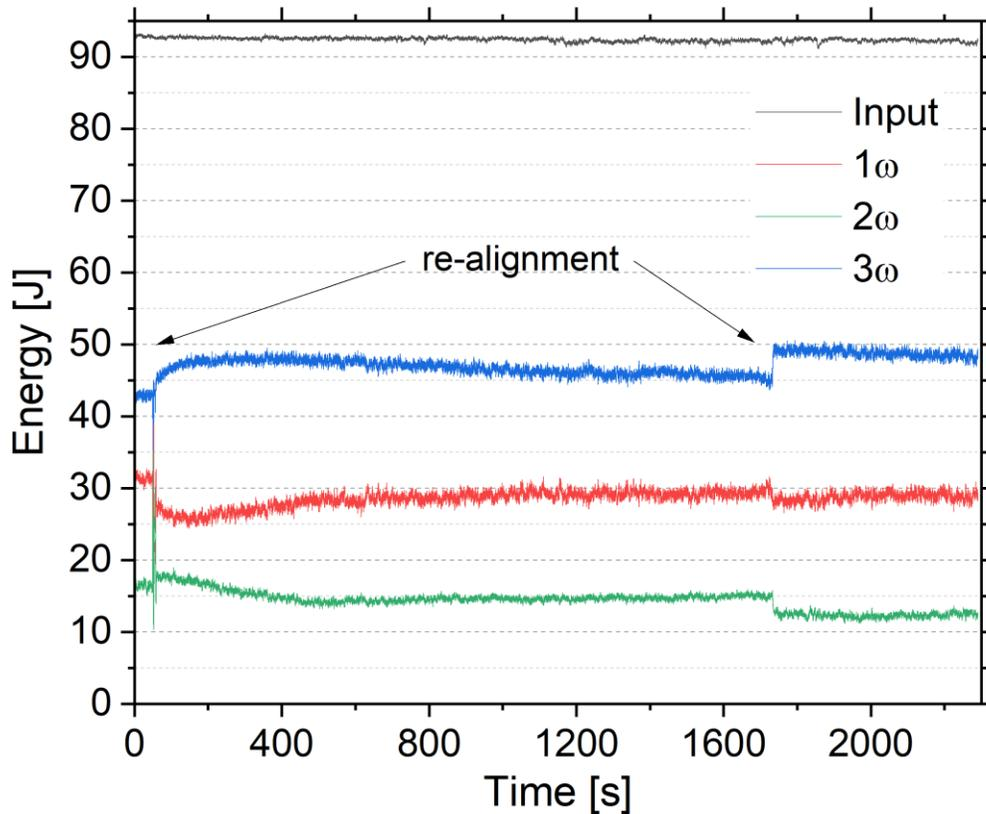
Figure 5 Temporal evolution of the energy of the third harmonic frequency  $3\omega$  (343 nm) together with input energy (1030 nm) and unconverted residual energy on fundamental  $1\omega$  (1030 nm) and second harmonic  $2\omega$  (515 nm) frequencies after SHG oven temperature stabilization.
