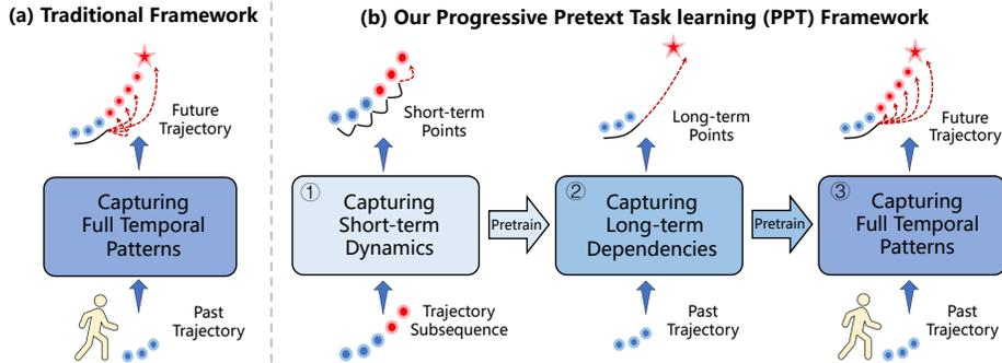
**Fig. 1:** Comparing our Progressive Pretext Task learning (PPT) framework with regular trajectory prediction. (a) Existing works tend to aggressively force the model to learn complicated full temporal patterns at once. (b) Our Framework employs three learning stages to progressively enhance the model for future trajectory prediction.
