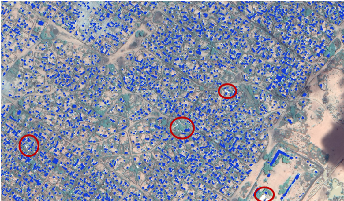
Figure 16: Predicted masks of FPN-MiT trained on Train-Small dataset without upscaling in Dagahaley Refugee Camp.
