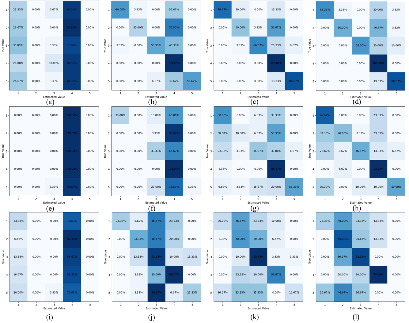
Fig. 4: Confusion matrices for within-session (a–d), cross-session (e–h), and randomized cross-session (i–l) experiments summed over the three subjects for: 0-shot (a, e, and i), 1-shot (b, f, and j), 2-shot (c, g, and k), and 3-shot (d, h, and l) strategies.
