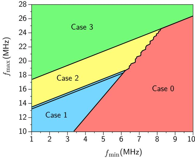
FIG. 5: Contour plots of the feasible frequency ranges for non-swap configurations, using ESA orbits ‘op25\_340\_10y3t.xyz’ (10 years). The boundary between case 0 and case 1 as well as between case 2 and case 3 (bold lines) is independent of the configuration, whereas the boundary between case 1 and case 2 (thin lines) depends on the configuration and choice of primary laser.
