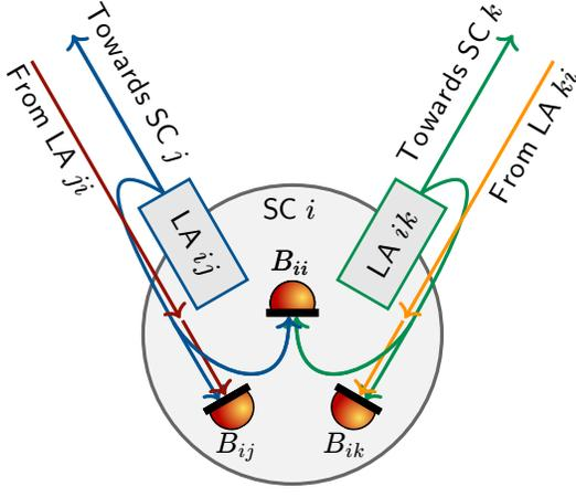
FIG. 2: Nomenclature used to enumerate spacecraft (SC), laser assemblies (LA), and beatnotes. In SC  $i$ , LA  $ij$  and LA  $ik$  are interfered to form the “local” beatnote  $B_{ii}$ . In addition, SC  $i$  receives the beams transmitted from the remote LA  $ji$  and LA  $ki$ , which are interfered with the local lasers to form the inter-spacecraft beatnotes  $B_{ij}$  and  $B_{ik}$  respectively.
