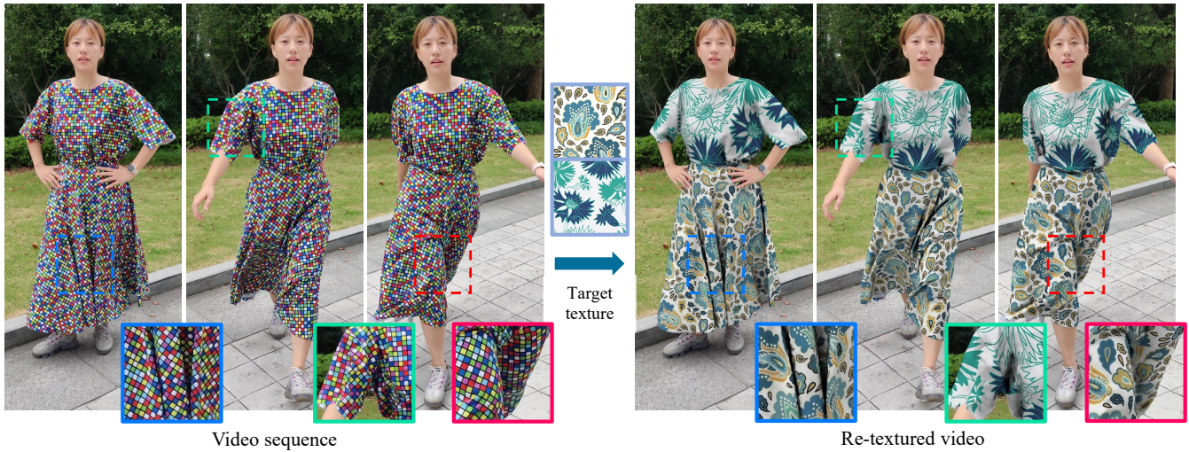
Fig. 1. We present an approach for pattern guided garment texture replacement in product virtual showcase. Given a video of a person wearing the target garments fabricated with our designed patterns, our method automatically extracts per-pixel UV coordinates for the garments in each frame as well as the shading and mask layers so that different texture maps can be applied to the image space for fast realistic visualization with just one click. The quality of our results lives up to the requirements from commercial applications where challenging areas such as folding areas and seams are nicely handled.
