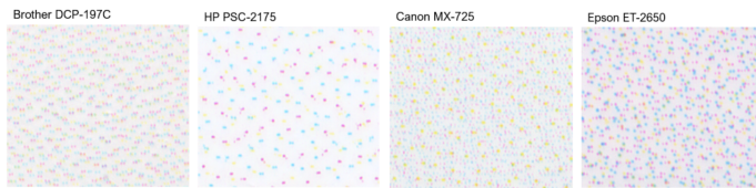
Fig. 3. Close view of inkjet printed documents. It is immediately recognizable that individual printer models produce distinct droplet patterns.
