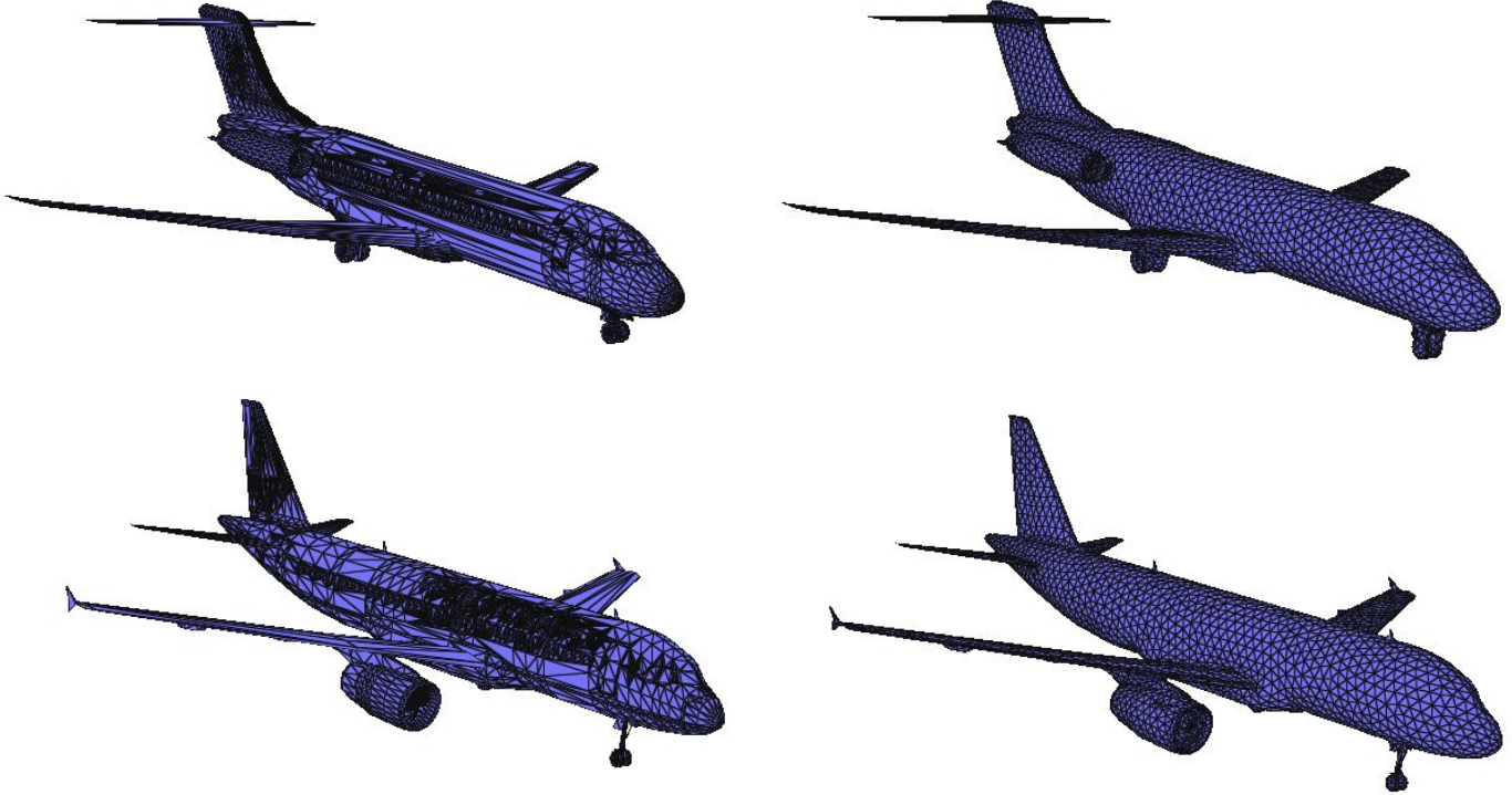
Fig. 1. Data pre-processing step for ShapeNet meshes. The left column contains the original meshes that are not watertight and have poor-quality triangulation. The meshes in the right column show the remeshing product.
