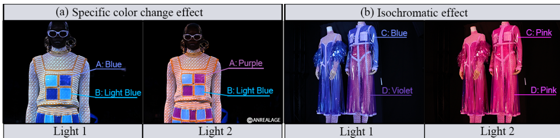
Figure 1: Our system has two technical contributions, which are visual effects that change the color appearance of objects by controlling the distribution of the illumination spectrum. (a) Specific color change effect: Comparing the color appearance of the dress under Light 1 and Light 2, the color of material A changes significantly, while material B remains its color, even after switching from Light 1 to Light 2. (b) Isochromatic effect: Materials C and D appear to be different colors under Light 1, while they appear to be the same color under Light 2. In both cases, we achieved designing Light 1 and Light 2 as a natural white appearance.
