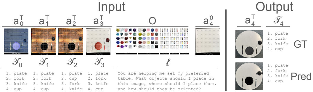
Figure 1: DegustaBot takes in a single person’s preferred table arrangements (shown here as the visual context k_i and order of object placement \mathcal{T}_i ), the objects O from which the algorithm can select, the table to set a_0 and the task prompt \ell . The robot then produces a task plan in the form of an object arrangement (visualized as an image a_T ) and the order of object placement \mathcal{T} . This predicted arrangement, Pred, should match a held-out preference created by the user, GT.
