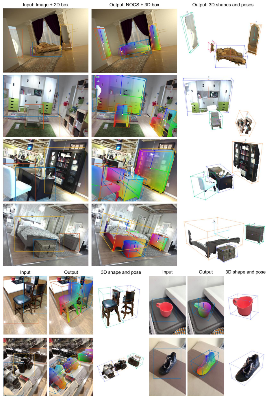
Fig. 9: Qualitative results of NOCSformer model for various indoor datasets. Left column shows the input images and query 2D bounding boxes. The center image shows the predicted per object NOCS, segmentation, and 3D oriented bounding box from our model corresponding to each input query overlaid on the input image. The right image shows the object coordinates lifted to 3D using the predicted 6DoF pose.
