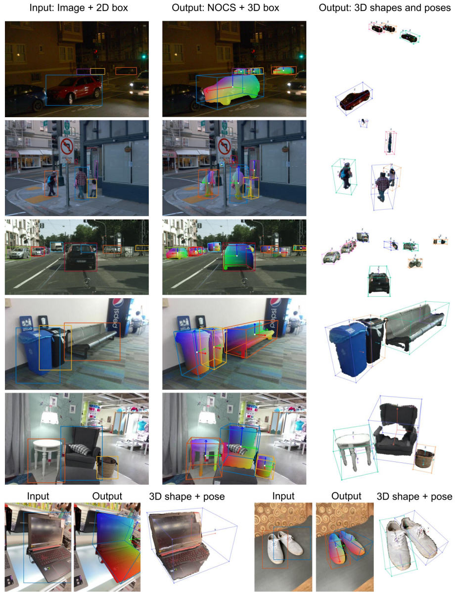
Fig. 4: Example results of our single unified NOCSformer model across various datasets and object classes. The left column shows input images and query 2D bounding boxes. The center column shows the NOCS+instance maps predicted by NOCSformer along with the estimated 3D pose overlaid on the input image. The NOCS can be used with the 3D boxes and object size to lift the objects to a 3D pointcloud, which is shown in the right column. Last row contains two examples.
