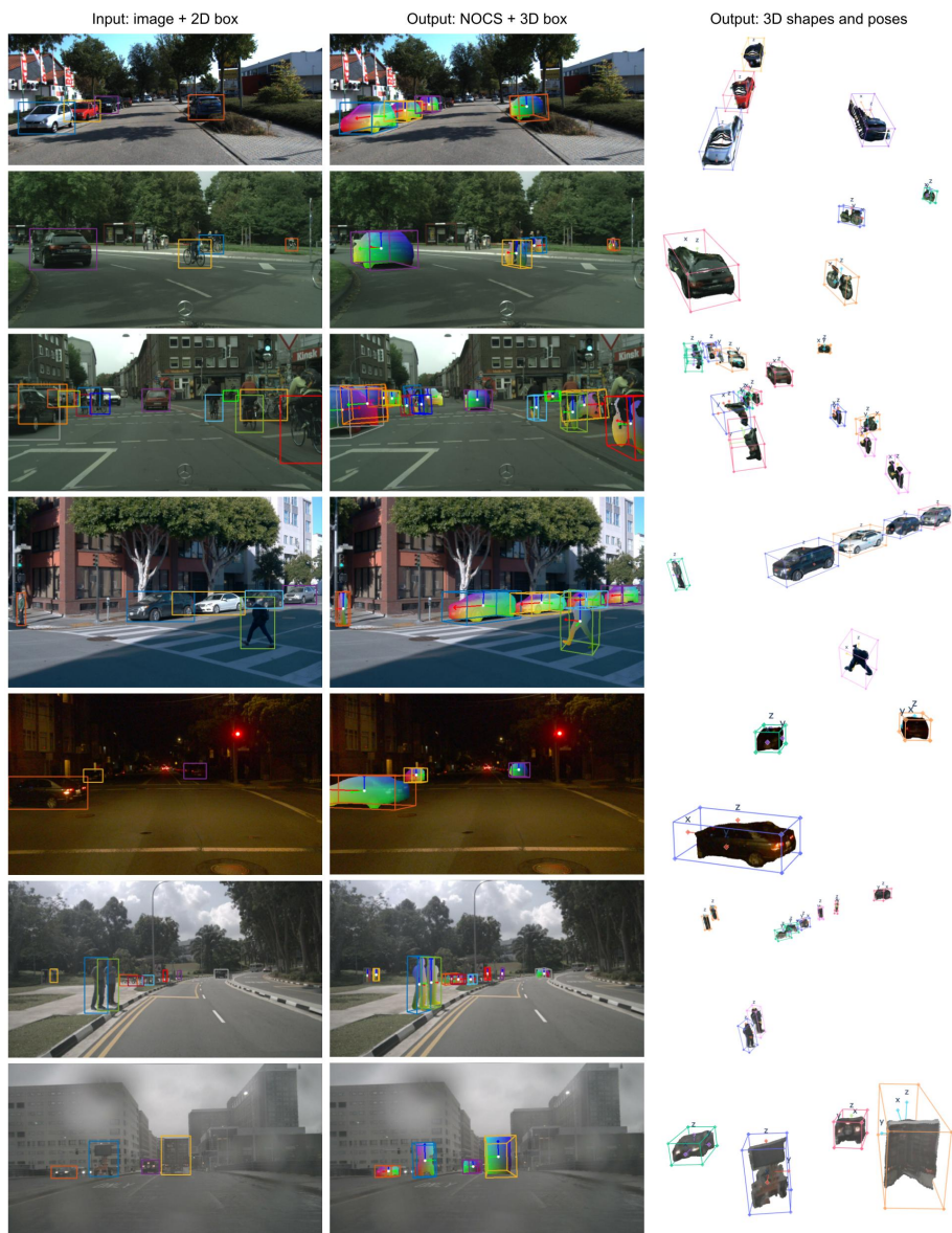
Fig. 8: Qualitative results of NOCSformer model for various outdoor datasets. Left column shows the input images and query 2D bounding boxes. The center image shows the predicted per object NOCS, segmentation, and 3D oriented bounding box from our model corresponding to each input query overlaid on the input image. The right image shows the object coordinates lifted to 3D using the predicted 6DoF pose.
