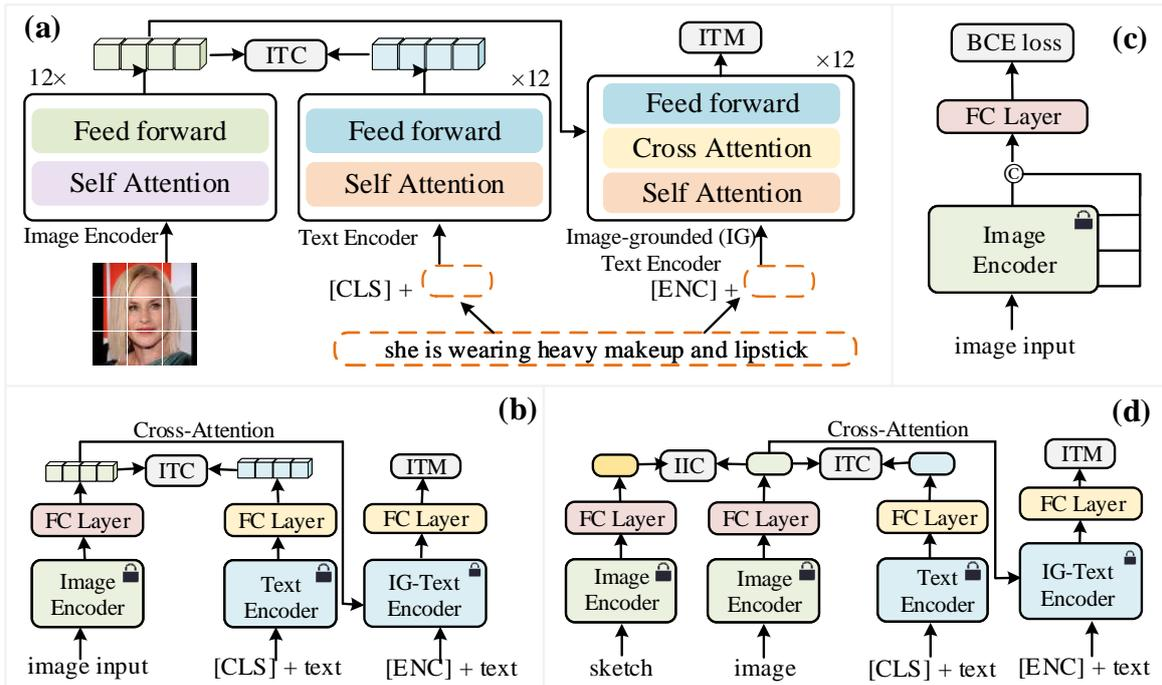
**Fig. 6:** Overview of FLIP architecture (a). Same color represents shared parameters. “12x” stands for 12-layer transformer modules. (b), (c) and (d) FLIP-based model are applied to the tasks of text-image retrieval, facial attributes prediction and sketch less facial image retrieval, respectively.
