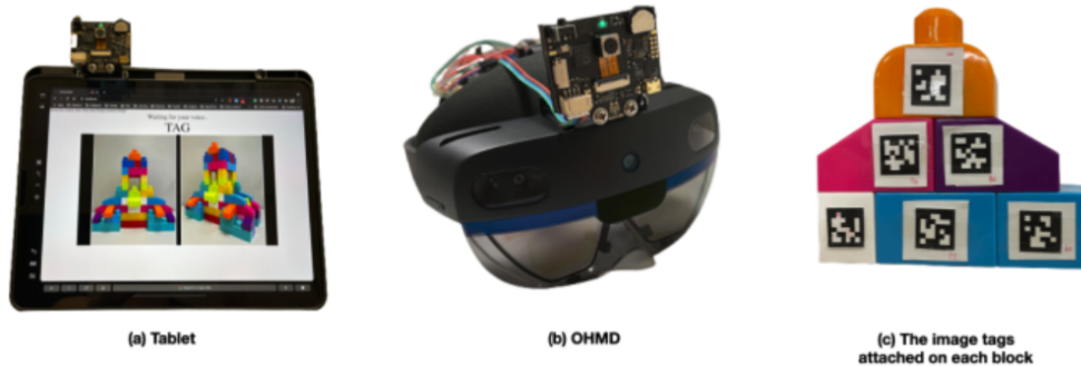
Figure 6: Prototyping: We mounted the HuskyLens Pro camera sensor [12] on both (a) a tablet and (b) an OHMD to recognize (c) unique image tags assigned to each toy-assembly block. This sensor is capable of identifying the pre-assigned ID numbers of the image tags when presented by the user. Upon identification, the sensor relays these ID numbers to the connected device—either the tablet or the smart glasses—via the Wi-Fi module of the accompanying Arduino board. The transmitted ID numbers are then used to update the displayed instructions on the device.
