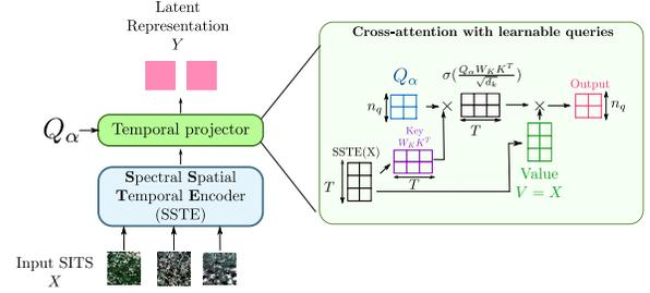
Figure 2. Overall description of ALISE architecture. The input time series  $X$  is first processed by the spectral spatial temporal encoder (SSTE). The obtained intermediate representations is then processed by a temporal projector. The temporal projector corresponds to a cross-attention mechanism with learnable queries  $Q_\alpha$ .
